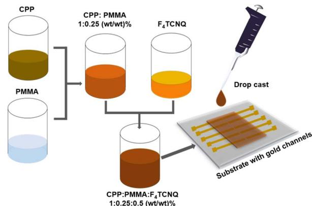
Fig. 5 Processability of CPPs is enhanced by blending them with insulating polymers; CPP : PMMA :  $F_4TCNQ$  (1 : 0.25 : 0.5) was blended in chlorobenzene and the resultant solution was drop cast into a thin film on top of a prefabricated chip with gold channels for conductivity measurements.
