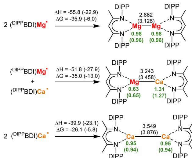
Scheme 2 Formation of homo- and hetero-metallic (<sup>DIPP</sup>BDI)Ae–Ae(<sup>DIPP</sup>BDI) complexes (Ae = Mg or Ca). Enthalpies and Gibbs free energies at 298 K in kcal mol<sup>-1</sup>, Ae–Ae distances in Å and NPA charges in green; B3PW91/def2TZVP//def2SVP with dispersion correction (GD3BJ). Values in brackets relate to calculations without dispersion corrections.
