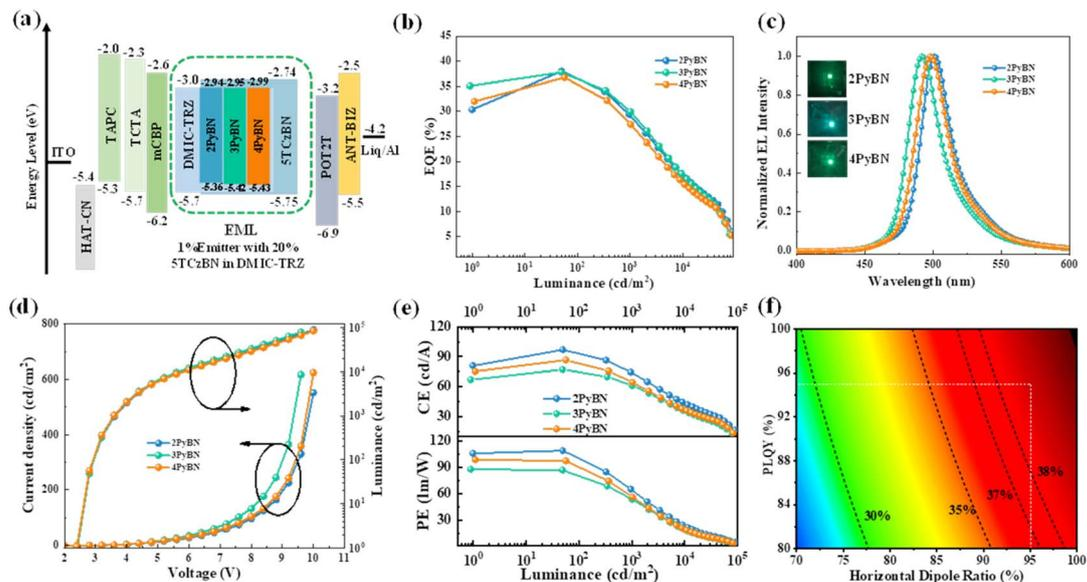
Fig. 4 (a) Device configuration and the energy level diagrams, (b) EQE versus luminance curves, (c) the EL spectra recorded at  $1000 \text{ cd m}^{-2}$  and the images of the devices, (d) luminescence and current density versus voltage characteristics, (e) CE/PE versus luminance curves, and (f) theoretical device efficiency with respect to PLQY and horizontal orientation factor via optical simulation.
