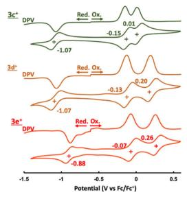
Fig. 5 CV and DPV of  $3c^+$ – $3e^+$  containing 0.1 M  $^n$ Bu<sub>4</sub>NPF<sub>6</sub> in CH<sub>2</sub>Cl<sub>2</sub> at a scan rate of 100 mV s<sup>-1</sup> ([ $3c^+$ – $3e^+$ ] = 1.0 mM).
