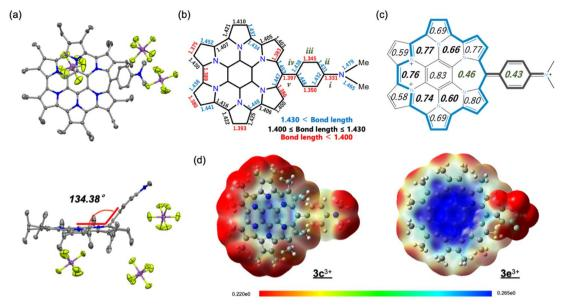
Fig. 7 (a) Crystal structures (top and side views) of  $3c^{3+}[SbF_6^-]_3$ . Thermal ellipsoids are scaled to 50% probability. Solvent molecules and disordered atoms are omitted for clarity. (b) Selected bond lengths (Å) and (c) HOMA values of the crystal structure of  $3c^{3+}[SbF_6^-]_3$ . (d) ESP plots of  $3c^{3+}$  and  $3e^{3+}$  calculated at the B3LYP/6-31G(d) level of theory, in which the Et groups are replaced with Me groups to simplify the calculations.
