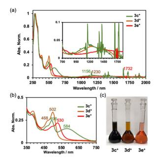
Fig. 4 (a) Absorption spectra of  $3c^+-3e^+$  in  $CH_2Cl_2$ , (b) enlarged view of the spectra in the visible light region, and (c) photographs of the solutions ( $[3c^+-3e^+] = 2.1 \times 10^{-5}$  M in  $CH_2Cl_2$ ).
