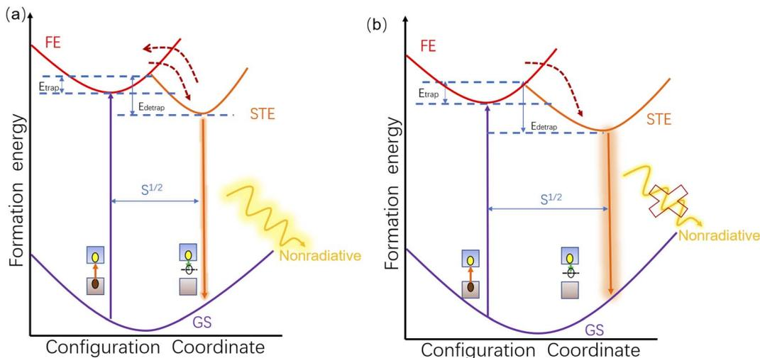
Fig. 5 (a and b) Illustration of the evolution of self-trapped exciton emission of the  $(2\text{mepth}_2)\text{PbCl}_4$  crystal at ambient conditions and 5.0 GPa. GS: ground state; FE: free exciton state; STE: self-trapped exciton state,  $E_{\text{trap}}$ : exciton trapping activation energy,  $E_{\text{detrapp}}$ : exciton detrapping activation energy,  $S$ : Huang–Rhys factor.
