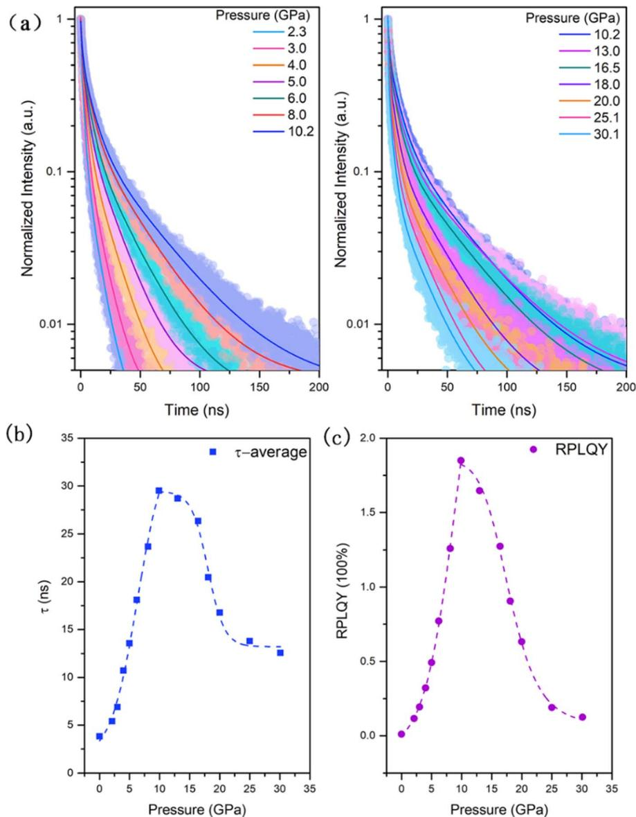
Fig. 4 (a) Normalized time-resolved PL decay curves of the  $(2\text{meptH}_2)\text{PbCl}_4$  crystal at selected pressure. (b) Average PL lifetime of  $(2\text{meptH}_2)\text{PbCl}_4$  as a function of pressure. (c) Evolution of estimated RPLQY during compression.
