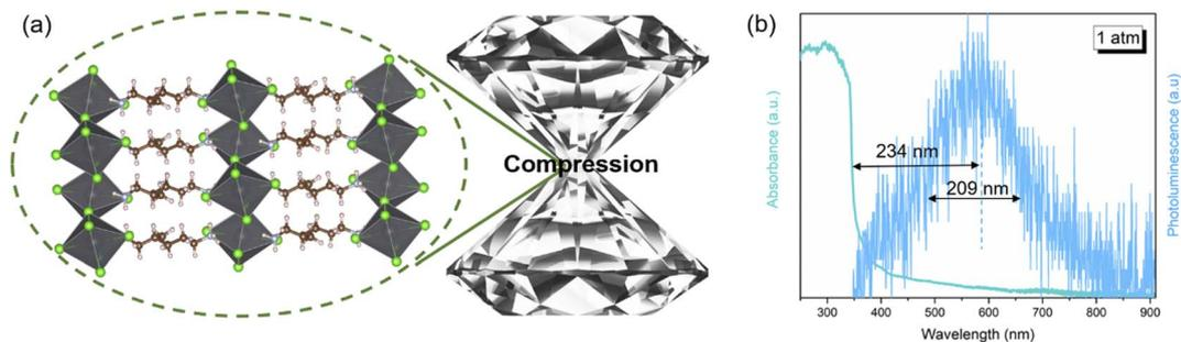
Fig. 1 (a) Ambient crystal structure of  $(2\text{mepH}_2)\text{PbCl}_4$  and simple schematic diagram of the diamond anvil cell used for high pressure experiments. (b) Absorption (turquoise) and photoluminescence (deep sky-blue) spectra excited by 355 nm ultraviolet light of  $(2\text{mepH}_2)\text{PbCl}_4$  crystals at ambient conditions.
