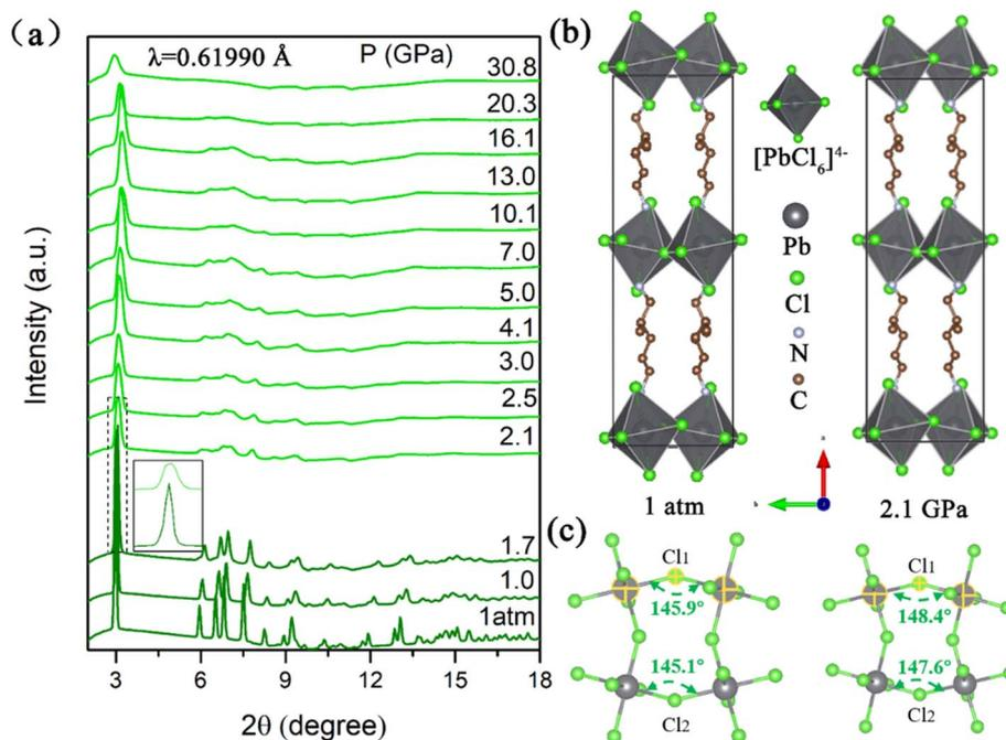
Fig. 3 (a) Representative *in situ* high-pressure ADXRD patterns of the  $(2\text{meptH}_2)\text{PbCl}_4$  crystal. (b) Crystal structure of  $(2\text{meptH}_2)\text{PbCl}_4$  perpendicular to the  $c$  axis. (c) Illustrations of the inorganic layer distortion at 1 atm and 2.1 GPa.
