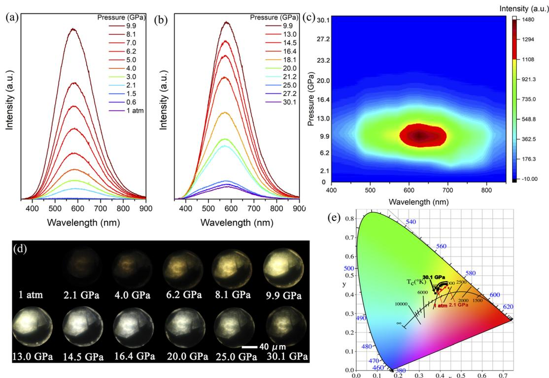
Fig. 2 (a and b) Pressure-induced evolution of emission spectra of  $(2\text{mepH}_2)\text{PbCl}_4$  upon compression; (c) two-dimensional projection of the PL emission spectra under compression; (d) optical images at selected pressures under UV irradiation of 355 nm; (e) chromaticity coordinates of the emissions as a function of pressure. The pressure range from 1 atm to 2.1 GPa is represented by the crimson round dots, while the range of 3.0–30.1 GPa is represented by the black diamond dots.
