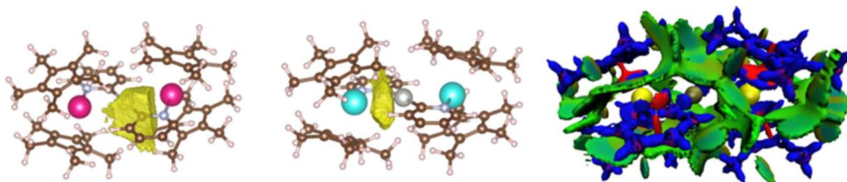
Fig. 7 Electronic density analysis of the trimetallic complexes: the ELF basin of **4** showing the Pd–C<sub>pyr</sub> interaction (left), basin corresponding to a Yb–Pd interaction on **5** (center) and DORI plot of **4** (right). Color-codes for the DORI plot: repulsive forces – red, covalent interaction – blue, and non-covalent interaction – green.
