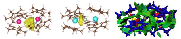
Fig. 7 Electronic density analysis of the trimetallic complexes: the ELF basin of 4 showing the  $Pd-C_{pyr}$  interaction (left), basin corresponding to a Yb-Pd interaction on 5 (center) and DORI plot of 4 (right). Color-codes for the DORI plot: repulsive forces – red, covalent interaction – blue, and non-covalent interaction – green.
