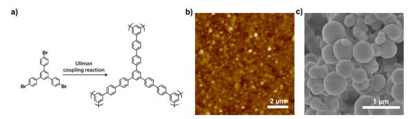
Fig. 5 (a) The chemical structure of PAF-5 and the corresponding synthetic routine; (b) AFM scan of PS/PAF-5; (c) SEM image of PAF-5 formed simultaneously in solution.
