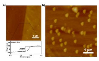
Fig. 4 (a) AFM scan of polymer brushes with low grafting densities grown on mixed SAMs and the corresponding sectional view; (b) AFM scan of PAF-1 grown on the brushes.
