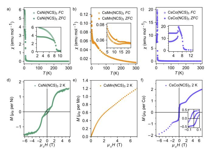
Fig. 2 Magnetic susceptibility data with an applied field of 0.01 T for (a) CsNi(NCS)<sub>3</sub>; (b) CsMn(NCS)<sub>3</sub>; (c) CsCo(NCS)<sub>3</sub>; and isothermal magnetisation measurements at 2 K for (d) CsNi(NCS)<sub>3</sub> (field –6 to +6 T); (e) CsMn(NCS)<sub>3</sub> (field 0 to +7 T); and (f) CsCo(NCS)<sub>3</sub> (field –7 to +7 T).
