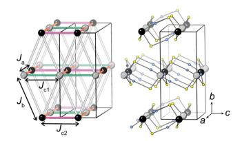
Fig. 5 The four nearest-neighbour magnetic interactions in CsM(NCS)<sub>3</sub>. M1 and M2 are grey and black respectively and the thiocyanate ligands are represented with sulfur (yellow) and nitrogen (blue) atoms only. Caesium cations and carbon atoms have been removed for clarity.
