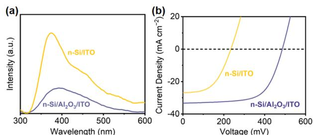
Fig. 4 (a) PL spectra and (b) solid-state  $J$ - $V$  characteristics of n-Si/ITO and n-Si/Al<sub>2</sub>O<sub>3</sub>/ITO.
