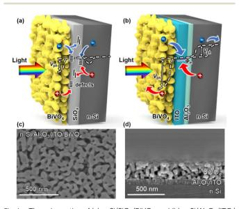
Fig. 1 . The schematics of (a) n-Si/SiO $_x$ /BiVO $_4$  and (b) n-Si/Al $_2$ O $_3$ /ITO/BiVO $_4$  integrated tandem photoanodes. The scanning electron microscopy images of (c) the surface morphology and (d) cross sections of the n-Si/Al $_2$ O $_3$ /ITO/BiVO $_4$  integrated tandem photoanode.
