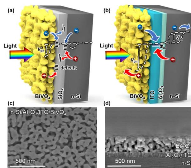
Fig. 1 The schematics of (a) n-Si/SiO<sub>x</sub>/BiVO<sub>4</sub> and (b) n-Si/Al<sub>2</sub>O<sub>3</sub>/ITO/BiVO<sub>4</sub> integrated tandem photoanodes. The scanning electron microscopy images of (c) the surface morphology and (d) cross sections of the n-Si/Al<sub>2</sub>O<sub>3</sub>/ITO/BiVO<sub>4</sub> integrated tandem photoanode.
