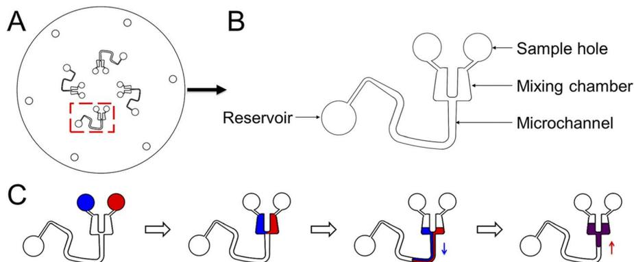
Fig. 2 The design of the CD microfluidic chip and illustration of the mixing process. (A) Illustration of the whole CD chip. (B) Illustration of one of the channels for mixing liquid. (C) The reciprocating motion of liquid in the modified microchannel. The blue arrow represents the direction of centrifugal force. The red arrow represents the direction of capillary force.
