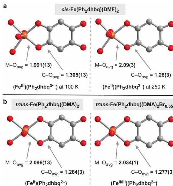
Fig. 3 (a) Coordination mode and average bond lengths in Å from the single crystal structures of  $cis-Fe(Ph_2dhubq)(DMF)_2$  at both 100 and 250 K. (b) Coordination mode and average bond lengths in Å from the single crystal structures of  $trans-Fe(Ph_2dhubq)(DMF)_2$  (undoped) versus  $trans-Fe(Ph_2dhubq)(DMF)_2Br_{0.55}$  (oxidatively doped), both at 250 K.
