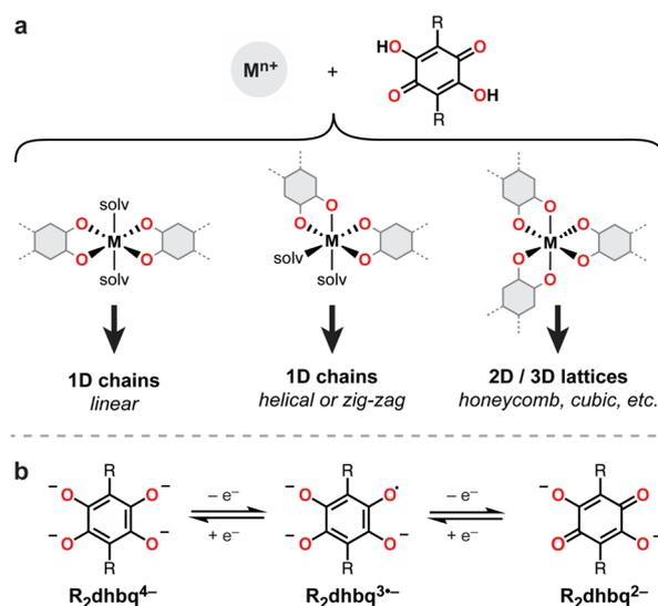
Fig. 1 (a) Binding modes for  $\text{H}_2\text{R}_2\text{dwbq}$  ligands and the resulting metal–organic structures. (b) Redox series of  $\text{R}_2\text{dwbq}^{7-}$  ligands. The ligand contains a radical in the  $\text{R}_2\text{dwbq}^{5\cdot-}$  state.
