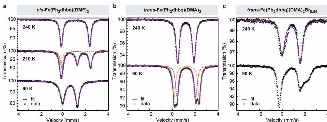
Fig. 4 Variable-temperature Mössbauer spectra of (a) *cis*-Fe(Ph<sub>2</sub>dhbq)(DMF)<sub>2</sub>, (b) *trans*-Fe(Ph<sub>2</sub>dhbq)(DMA)<sub>2</sub>, and (c) *trans*-Fe(Ph<sub>2</sub>dhbq)(DMA)<sub>2</sub>Br<sub>0.55</sub>. Experimental data are represented as individual black crosses, fits for individual doublets within each spectrum are represented by dashed lines, and the overall fit for each spectrum is represented by a solid line.
