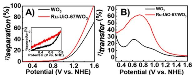
Fig. 5 (A) Charge separation efficiency ( $\eta_{sep}$ ) of  $WO_3$  (black) and  $Ru-UiO-67/WO_3$  (red) films; inset shows the same figure but magnified from 0.2 to 0.8 V vs. NHE. (B) Charge transfer efficiency ( $\eta_{trans}$ ) for  $WO_3$  (black) and  $Ru-UiO-67/WO_3$  (red) films. Addition of  $Ru-UiO-67$  to  $WO_3$  improves charge separation and charge transfer within  $WO_3$  at the electrode surface over all applied potentials.
