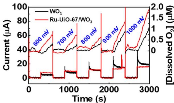
Fig. 8 Current increase (bottom) and O<sub>2</sub> production (top) for WO<sub>3</sub> and Ru-UiO-67/WO<sub>3</sub> at different applied potentials. At each potential, the photoelectrode was held in the dark for 5 minutes before illumination for 5 minutes.
