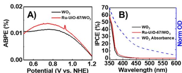
Fig. 3 (A) Photo-response efficiency of WO<sub>3</sub> (black) and Ru-UiO-67/WO<sub>3</sub> (red) as a function of potential (ABPE). (B) Wavelength (IPCE) of WO<sub>3</sub> (black), Ru-UiO-67/WO<sub>3</sub> (red) measured under monochromatic light at 500 mV applied potential, overlaid WO<sub>3</sub> absorption spectrum (blue dashed line).
