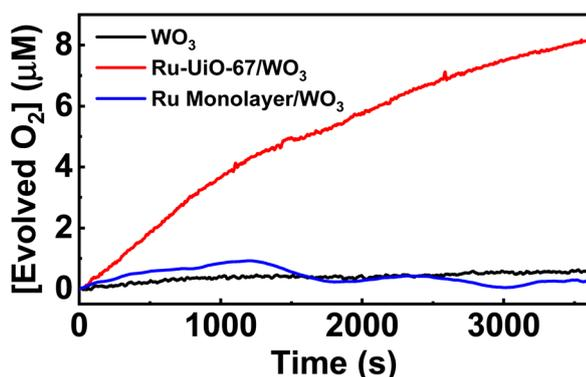
Fig. 9 Oxygen production of Ru-UiO-67/WO<sub>3</sub> over time, compared to bare WO<sub>3</sub>. Ru-UiO-67/WO<sub>3</sub> activity was averaged across three different films (Fig. S13†).
