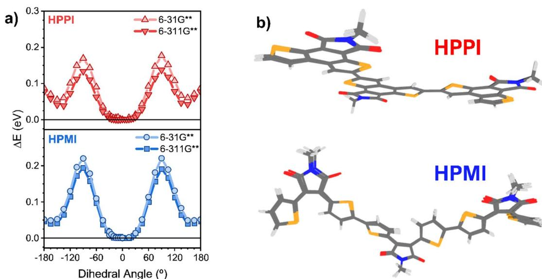
Fig. 2 (a) Relaxed potential energy scan around the Se–C–C–Se dihedral bond performed with B3LYP/6-31G\*\* and B3LYP/6-311G\*\*. The y axis,  $\Delta E$ , is the energy relative to the global minimum. (b) Superimposed ground state optimised geometries calculated at the levels of theory B3LYP/6-31G\*\*, B3LYP/6-311G\*\*, CAM-B3LYP/6-31G\*\*, CAM-B3LYP/6-311G\*\* and  $\omega$ B97X-D3/6-31G\*\* of HPPI (top) and HPMI (bottom) trimers.
