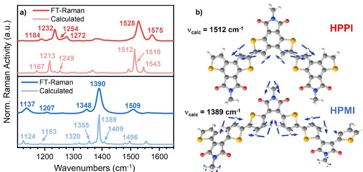
Fig. 3 (a) Comparison of the calculated (B3LYP/6-31G\*\*) (lighter lines) and experimental (darker lines) FT-Raman spectra for HPPI (top) and HPMI (bottom) films. (b) Eigenvectors of the vibrational modes corresponding to the most intense Raman band for HPPI and HPMI (experimentally seen at 1528 and 1390  $\text{cm}^{-1}$ , respectively).
