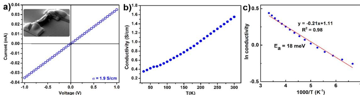
Fig. 6 (a)  $I$ - $V$  curve for two-contact probe single crystal measurement, (b) electrical conductivity of **1** as a function of temperature, and (c) Arrhenius fitting of conductivity to temperature.
