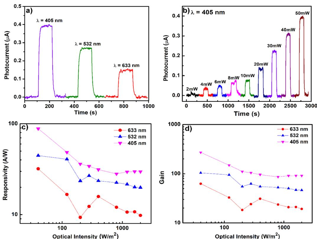
Fig. 7 (a) Photocurrent responses at excitation wavelengths of  $\lambda = 405$ , 532, and 633 nm, (b) a time-dependent photocurrent response at  $\lambda = 405$  nm at different optical powers, (c) responsivity, and (d) photoconductive gain at the different excitation wavelengths.
