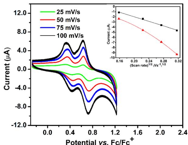
Fig. 3 Scan rate dependent cyclic voltammetry of **1** at scan rates from 25 mV s<sup>-1</sup> to 100 mV s<sup>-1</sup>. Inset: plots of current vs. (scan rate)<sup>1/2</sup> for the first oxidation wave (black) and second oxidation wave (red).
