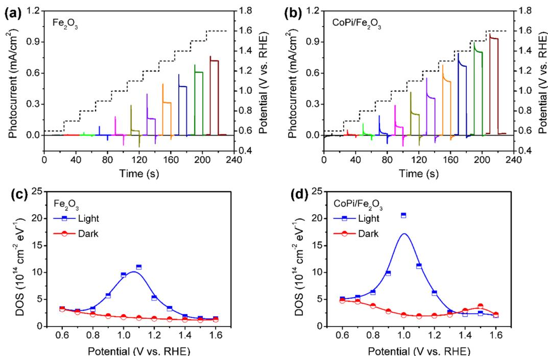
Fig. 1 Potential-dependent transient photocurrents for (a) bare Fe<sub>2</sub>O<sub>3</sub> and (b) CoPi/Fe<sub>2</sub>O<sub>3</sub> photoanodes under chopped illumination (AM 1.5 G: 100 mW cm<sup>-2</sup>). The applied potential is shown by a dashed line in the right axis. DOS of surface states in (c) bare Fe<sub>2</sub>O<sub>3</sub> and (d) CoPi/Fe<sub>2</sub>O<sub>3</sub> as a function of potential under illumination (456 nm LED: 5 mW cm<sup>-2</sup>) and in the dark.
