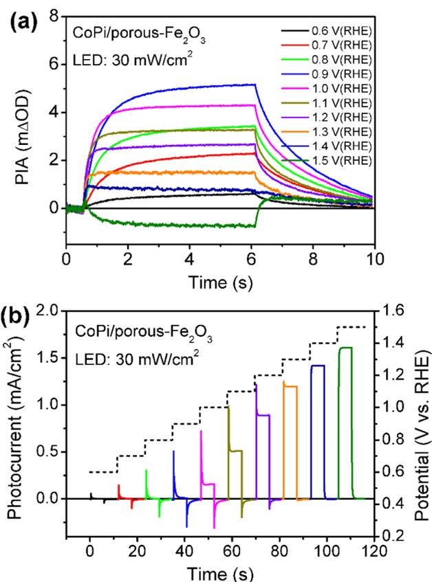
Fig. 4 Potential-dependent PIA spectra (a) and chopped photocurrents (b) for  $\text{CoPi}/\text{porous-Fe}_2\text{O}_3$ . Pump wavelength is 456 nm ( $30 \text{ mW cm}^{-2}$ ); probe wavelength is 694.3 nm; colors of curves at different potentials in (a) and (b) are identical.
