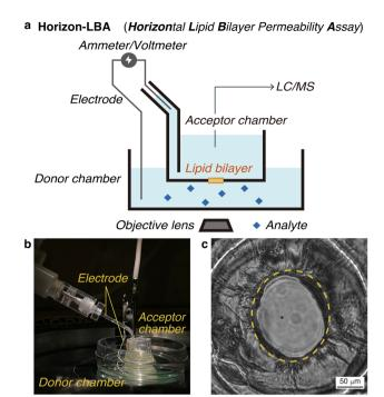
Fig. 2 Horizontal lipid bilayer permeability assay (Horizon-LBA). (a) Schematic illustration of the entire assay system. (b) A side view of the system. (c) A picture of the lipid bilayer constructed in the pore at the bottom of the acceptor chamber. The yellow circle indicates a lipid bilayer on the pore.
