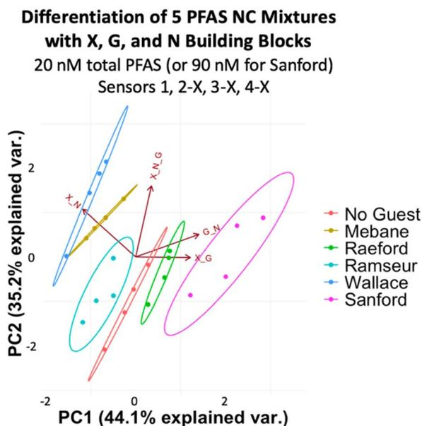
**Fig. 11** PCA plot displaying detection of five PFAS mixtures in 50 mM sodium borate buffer (pH 8.5) varying in components, ratios, and total concentration (according to Table 2) and a No Guest sample using sensors 1, 2-X, 3-X, and 4-X (G + N, X + G, X + N, and X + G + N DCLs) at 20 nM total PFAS (or 90 nM for the Sanford Sample). PCA plots are shown with 95% confidence ellipses.
