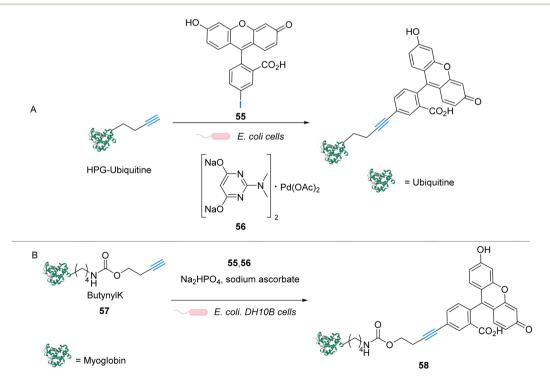
Fig. 23 (A) Copper-free Sonogashira cross-coupling reaction inside *E. coli* for fluorescent labelling of HPG-Ub protein by modified fluorescein using a discrete Pd<sup>II</sup> precatalyst. (B) Sonogashira cross-coupling labeling of Myoglobin inside *E. coli*.<sup>65,66</sup>
