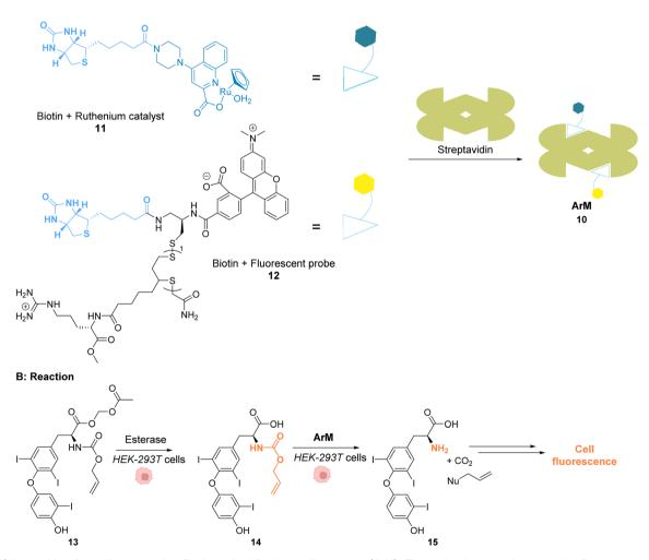
Fig. 5 (A) Assembly of a cell-penetrating Ru-based artificial metalloenzyme (ArM). The ruthenium catalyst and the fluorescent probe/cell penetrating peptide are both attached to biotin units interacting with streptavidin to create the artificial metalloprotein; (B) the ArM catalyses the Alloc deprotection of compound 14, generating the hormone 15. The HEK-293T cells have been modified to become fluorescent once 15 is liberated.40
