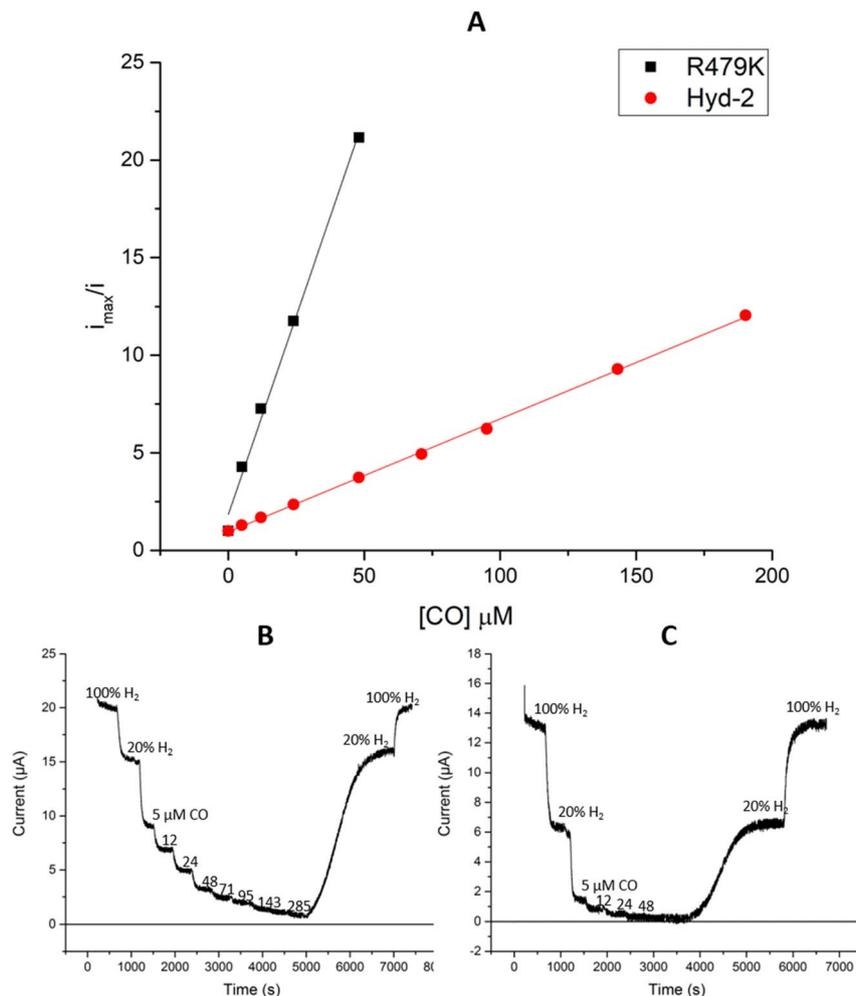
Fig. 5 Calculation of the  $K_i^{CO}$  (A) for Hyd-2 and R479K using the data from the profiles of inactivation in 20% H<sub>2</sub> in varying concentrations of CO for (B) Hyd-2 and (C) R479K. Other conditions: potential  $-0.175$  V,  $\omega = 3000$  rpm, 20 °C, pH 6.0, Ar carrier gas, total gas flow rate of 1000 sccm.
