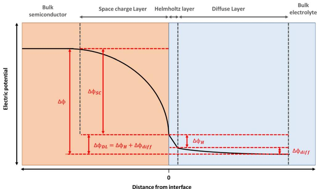
Fig. 1 Potential distribution at a typical n-type semiconductor|electrolyte junction, where  $\Delta\phi_{SC}$  represents the potential drop over the space charge layer,  $\Delta\phi_H$  over the Helmholtz layer and  $\Delta\phi_{diff}$  over the diffuse layer (such that the potential drop over the double layer,  $\Delta\phi_{DL} = \Delta\phi_H + \Delta\phi_{diff}$ ). The high electrolyte concentrations employed allow us to approximate  $\Delta\phi \sim \Delta\phi_H + \Delta\phi_{SC}$ .
