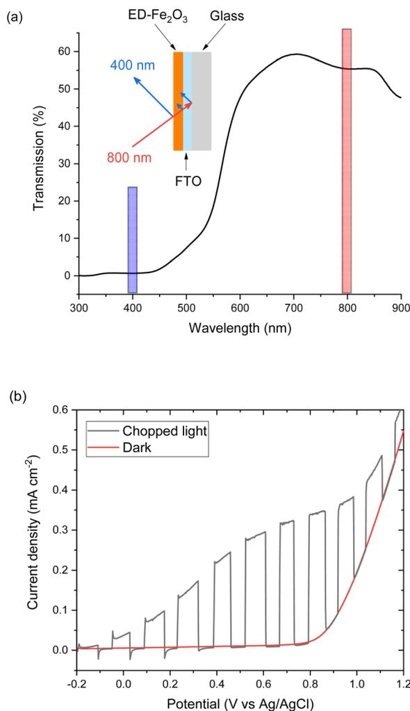
Fig. 2 (a) UV-vis in transmission of the  $\alpha$ -Fe<sub>2</sub>O<sub>3</sub> electrode used for SHG experiments. Inset, experimental geometry for reflection SHG experiments, highlighting the absorption of SHG photons (blue) from the buried interface by the layer of hematite on commercial FTO-coated glass. (b) Chopped light (15 mW cm<sup>-2</sup>, 365 nm) and dark linear sweep voltammograms (LSVs) at 10 mV s<sup>-1</sup> of  $\alpha$ -Fe<sub>2</sub>O<sub>3</sub> electrode in 0.1 M NaOH.
