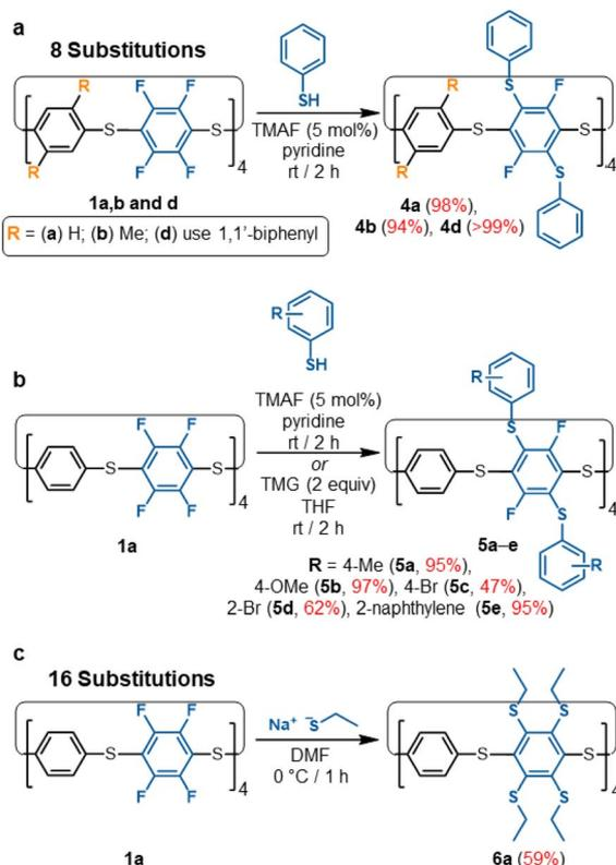
Scheme 2 (a) Synthesis of thiophenol functionalised  $S_8$ -corona[n]arenes (**4a**, **4b**, **4d**). (b) Scope of 8-fold functionalisation of **1a** to **5a–e**; (c) 16-fold functionalisation of **1a** to **6a**.
