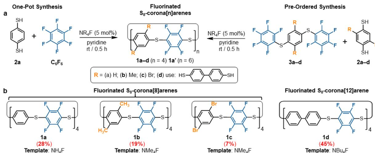
Scheme 1 (a) Two routes to synthesise fluorinated  $S_8$ -corona[ $n$ ]arenes (**1**): from  $C_6F_6$  and from analogues (**3**). (b) Schematic representations of macrocycles (**1a–d**) synthesised from the pre-ordered route, indicating the optimal  $NR_4F$  catalytic template.
