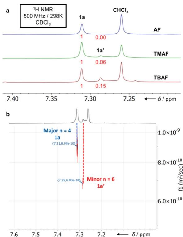
Fig. 2 Partial (a)  $^1\text{H}$  NMR spectra ( $\text{CDCl}_3$ ) of  $\text{S}_8$ -corona[8]arene (**1a**) and  $\text{S}_{12}$ -corona[12]arene (**1a'**) as synthesised via **3a** promoted by different ammonium fluoride catalysts. (b) Diffusion-Ordered Spectroscopy (DOSY) NMR spectrum of a **1a**:**1a'** mixture.
