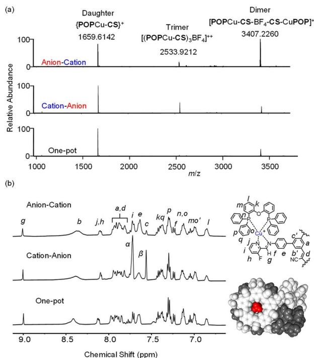
Fig. 9 (a) ESI-MS ( $\text{CH}_2\text{Cl}_2$ , 0.5 mM) and (b) diagnostic  $^1\text{H}$  NMR peaks ( $\text{CD}_2\text{Cl}_2$ , 0.5 mM) for  $[\text{POPCu-CS-BF}_4\text{-CS-CuPOP}]^+$  for the anion-cation stepwise, cation-anion stepwise, and one-pot assembly.
