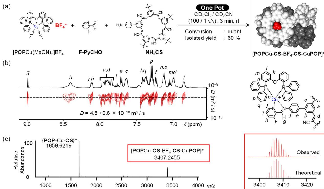
Fig. 3 (a) One-pot reaction to form  $[\text{POPCu-CS-BF}_4\text{-CS-CuPOP}]^+$  and characterization by (b) DOSY NMR ( $\text{CD}_2\text{Cl}_2$ , 2 mM), and (c) ESI-MS spectrum of assembly ( $\text{CH}_2\text{Cl}_2$ , 2 mM).
