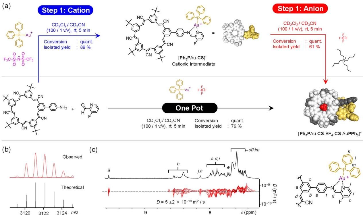
Fig. 12 (a) Reactions to form  $[\text{PPh}_3\text{Au-CS-BF}_4\text{-CS-AuPPh}_3]^+$  by one-pot and cation–anion pathways. (b) ESI-MS ( $\text{CH}_2\text{Cl}_2$ , 0.5 mM) of  $[\text{PPh}_3\text{Au-CS-BF}_4\text{-CS-AuPPh}_3]^+$  prepared via cation–anion pathway. (c) DOSY NMR ( $\text{CD}_2\text{Cl}_2$ , 2 mM) of  $[\text{PPh}_3\text{Au-CS-BF}_4\text{-CS-AuPPh}_3]^+$  created in one-pot assembly.
