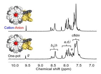
Fig. 13 Diagnostic  $^1H$  NMR peaks (CD<sub>2</sub>Cl<sub>2</sub>, 0.5 mM) for [PPh<sub>3</sub>Au-CS-BF<sub>4</sub>-CS-AuPPh<sub>3</sub>]<sup>+</sup> obtained by one-pot assembly and cation–anion assembly.
