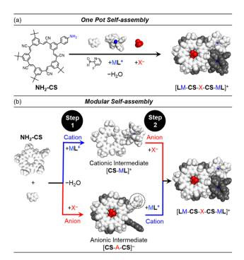
Fig. 1 Schematic summary of the (a) one-pot and (b) two-step selfassembly pathways that use pre-programmed and orthogonal coordination of cations and anions. In the resulting assembly (at right) the top cyanostar is shown in white and the bottom one is shown in dark grey for clarity. The Cu<sup>+</sup> cation is shown in blue, and the BF<sub>4</sub><sup>-</sup> anion shown in red. The pyridyl-based aldehyde is highlighted by the dotted circle in the anionic intermediate.
