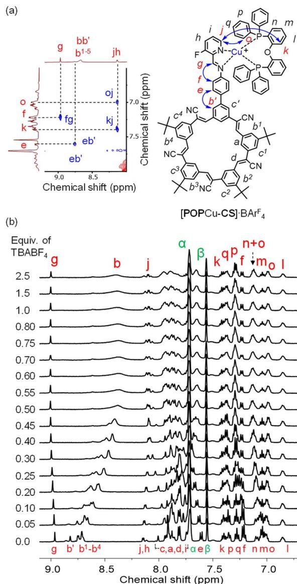
Fig. 6 (a) The aromatic region of ROESY NMR data of  $[\text{POPCu-CS}]^+\cdot\text{BARF}_4^-$ . (b)  $^1\text{H}$  NMR titration of  $[\text{CS-POPCu}]^+\cdot\text{BARF}_4^-$  (2 mM) with  $\text{TBABF}_4$  ( $\text{CD}_2\text{Cl}_2$ , 400 MHz, rt).
