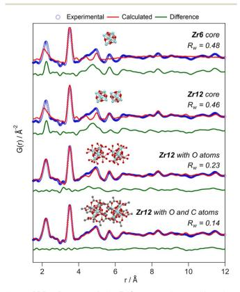
Fig. 4 PDF refinement of the **Zr12**-acetate cluster with various models, derived from the reported crystal structure.  $^4$  The best fit is obtained when including the oxygen and carbon atoms from the acetate ligands. The refined parameters are given in Table S1. $^{\dagger}$
