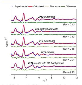
Fig. 5 PDF refinement for Zr12-butanoate and Zr12-octanoate using the Zr12-acetate structure model. PDF refinement of Zr6-methyl-butanoate using the Zr6-acetate structure model. Finally, the PDF refinement of Zr12-oleate using the Zr12-propionate structure model, with or without background correction in reciprocal space. If applied in the refinement, the exponentially dampening sine wave is shown (orange dotted lines). The refined parameters are given in Table S3.†
