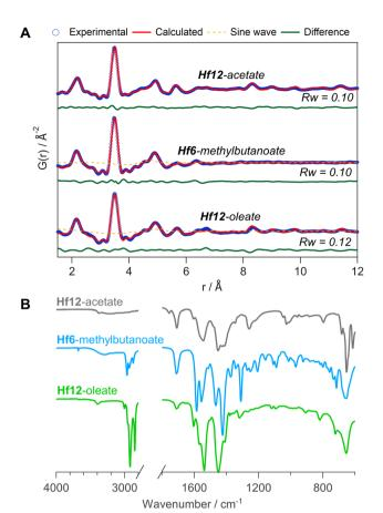
Fig. 10 (A) PDF fit for Hf12-acetate, Hf6-methylbutanoate and Hf12-oleate clusters with exponentially dampening sine wave contribution. The refined parameters are indicated in Table S9.† (B) FTIR spectra of the hafnium oxo clusters synthesized *via* bottom up.
