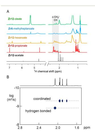
Fig. 7 (A) NMR spectra in  $CDCl_3$  of Zr12-acetate, -propionate, -hexanoate and -oleate and Zr6-methylheptanoate. (B) DOSY of the Zr12-acetate cluster with one faster diffusing species and a set of three resonances pertaining to a slowly diffusing species (the cluster).
