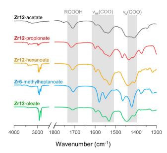
Fig. 6 FTIR spectra of Zr12-acetate, -propionate, -hexanoate, and -oleate and Zr6-methylheptanoate. The weak band at 1750 cm<sup>-1</sup> in the spectrum of Zr12-acetate is assigned to a small amount of acetic acid that is not involved in hydrogen bonding of any kind.<sup>71</sup> An ester impurity is ruled out because of the absence of any signal at around 4 ppm in NMR, (see Fig. S10†).
