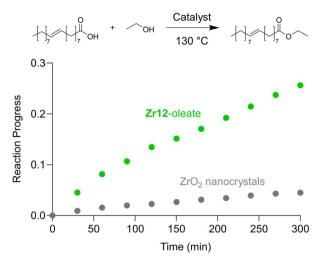
Fig. 11 Catalytic esterification of oleic acid with ethanol, catalyzed by either Zr12-oleate (green) or  $ZrO_2$  nanoparticles (gray). In both cases, 10 mol% Zr, with respect to the carboxylic acid substrate, was added.
