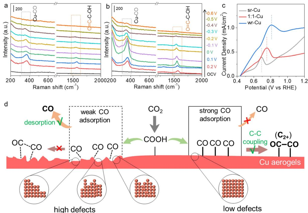
Fig. 3 The *in situ* Raman spectra for sr-Cu (a) and wr-Cu (b) aerogels at various potentials (vs. RHE) during the  $CO_2RR$ . OCV means open-circuit voltage. (c) The electrochemical CO stripping voltammetry test for sr-Cu, 1:1-Cu and wr-Cu aerogels in CO-saturated  $0.1\text{ M Na}_2SO_4$  solution. (d) Proposed structure–activity relationship diagram on different Cu aerogel surfaces: comparison of key steps in the  $C_1$  and  $C_{2+}$  reaction pathways.
