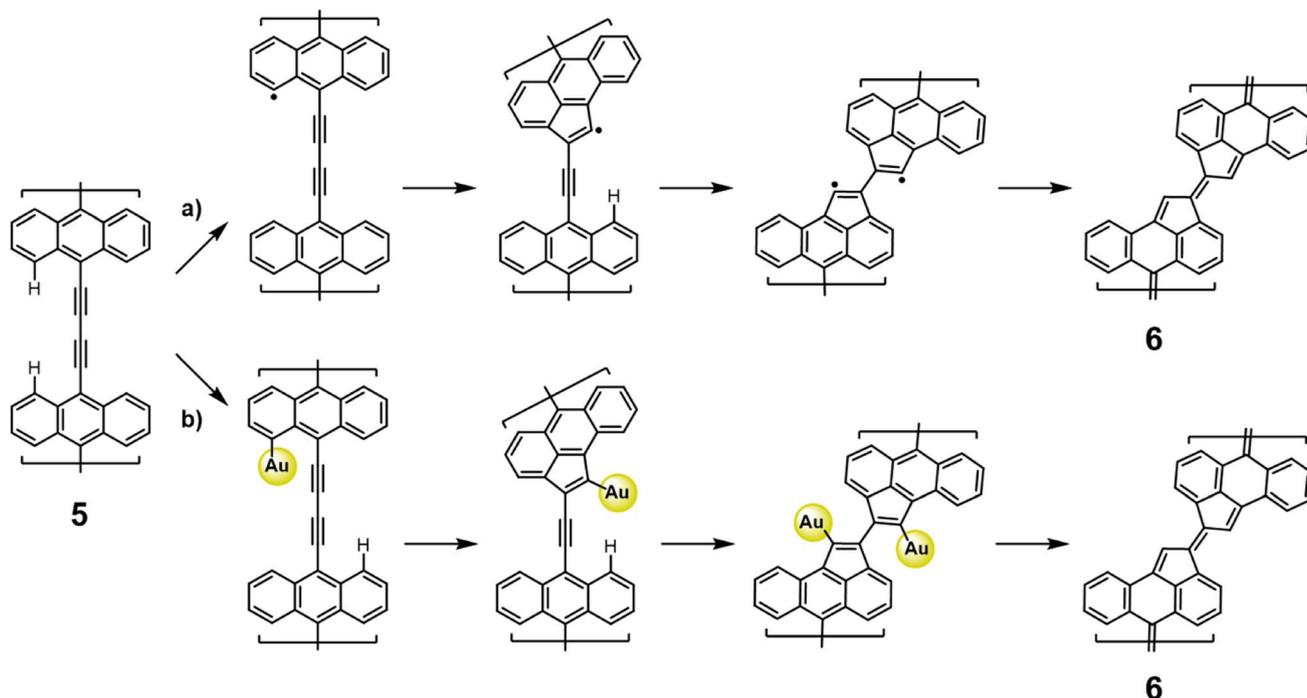
Fig. 3 Proposed reaction mechanism giving rise to fulvalene units. (a) Traditional, and (b) on-surface proposed ethynylarene rearrangement to cyclopenta fused polycyclic aromatic hydrocarbons. An initial hydrogen abstraction is followed by oxidative ring closure and  $\pi$ -electron reconfiguration, while individual gold atoms may stabilize transient radicals.
