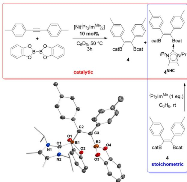
Scheme 3 Deactivation of the catalyst and independent synthesis of  $Z$ -(Bcat)(4-Me-C<sub>6</sub>H<sub>4</sub>)C=C(4-Me-C<sub>6</sub>H<sub>4</sub>)(Bcat)·(*i*Pr<sub>2</sub>Im<sup>Me</sup>) 4<sup>NHC</sup>. For selected bond lengths and angles in 4<sup>NHC</sup> see Fig. S17 in the ESI.†
