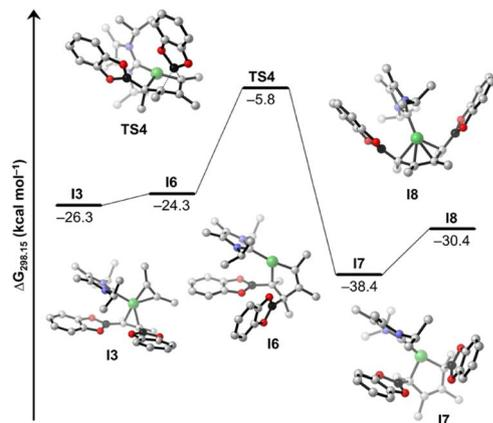
Fig. 6 Free energy profile of the proposed mechanistic pathway from **I3** to **I8**. Calculated free energies ( $\text{kcal mol}^{-1}$ ) are at the SMD(benzene)/PBE0-D3(BJ)/def2-TZVPP//PBE0-D3(BJ)/def2-SVP/def2-TZVP(Ni) level of theory, and are referenced to the resting state **14a** +  $\text{C}_2\text{Me}_2$  +  $\text{B}_2\text{cat}_2$ . Hydrogen atoms are omitted for clarity.
