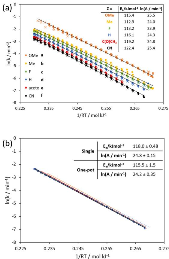
**Fig. 3** Arrhenius plots generated from transient temperature ramp experiments on: (a) a mixture of six substrates **1a–f** over two repeated (x and o) bi-directional temperature ramp experiments (170–250–170 °C) (OP-TF); (b) allyphenylether (**1d**) over different temperature ranges collected from a single substrate (IS-TF, full lines) and in the presence of 5 other substrates (OP-TF, dotted lines).  $E_a$  is the activation energy and  $A$  is the pre-exponential factor of the Hammett plot.
