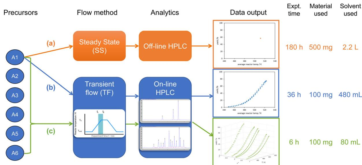
**Fig. 1** Comparison of different flow methods for collecting kinetic data: (a) individual substrate steady state flow (IS-SS); (b) individual substrate transient flow (IS-TF); and (c) one-pot transient flow (OP-TF). Estimated amount of experimental time, material, and reaction solvent required for each method to collect the same number of datapoints as the one-pot transient flow method.
