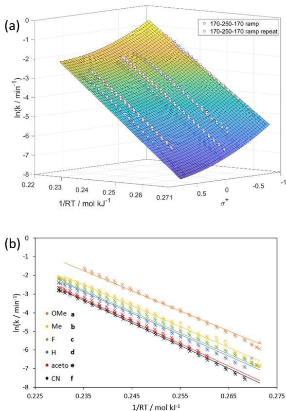
**Fig. 5** (a) “Arrhenius–Hammett model” surface with two bi-directional temperature ramping experiments (170–250–170 °C) generated from the six training substrates **1a–1f**; (b) comparison of experimental data (crosses) and model predictions (lines) of Arrhenius plots on the ‘training’ substrates **1a–1f**.
