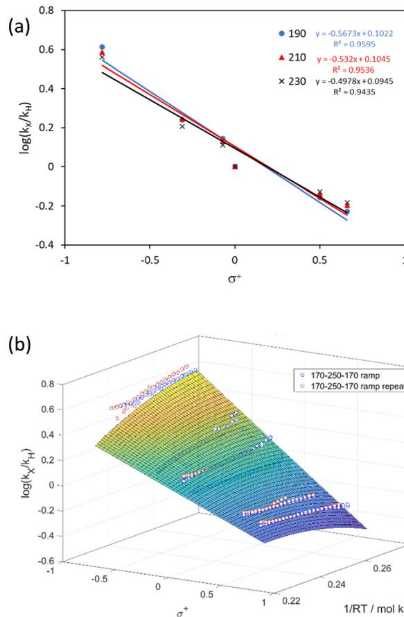
**Fig. 4** (a) Hammett plots at 190, 210 and 230 °C generated from OP-TF experiments; (b) temperature dependent Hammett plot visualizations of two 170–250–170 °C temperature ramping experiment on a mixture of six substrates **1a–f**. The surface fitting is first order in  $\sigma^+$  and second order in  $1/RT$ .
