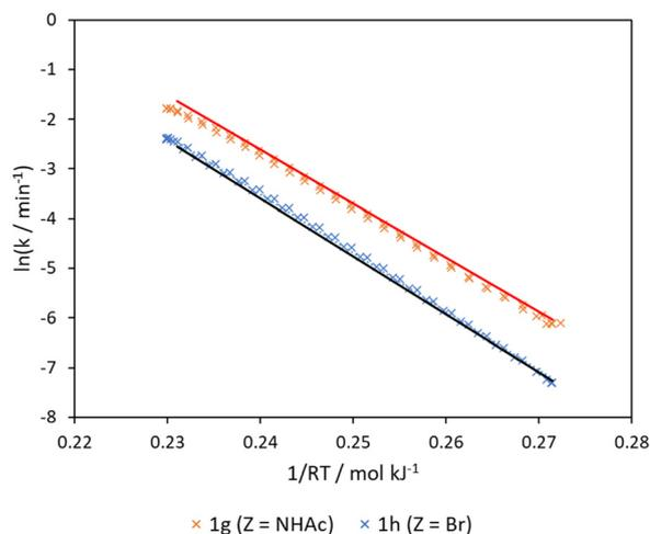
**Fig. 6** Arrhenius plots generated from bi-directional temperature ramp experiments (170–250–170 °C) (crosses) compared to Arrhenius–Hammett model predictions (lines) for phenyl allyl ether **1g** ( $Z = \text{NHAc}$ ) and **1h** ( $Z = \text{Br}$ ).
