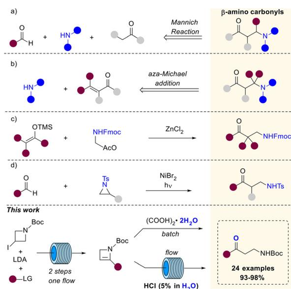
**Scheme 1** Preparation of  $\beta$ -aminocarbonyl compounds. a) Mannich-type reaction; b) aza-Michael addition; c)  $\text{ZnCl}_2$  catalyzed addition of carbon nucleophiles to Fmoc-protected *N,O*-acetals; d) photocatalyzed ring opening of *N*-tosyl styrenyl aziridines with aldehydes; bottom: this work.
