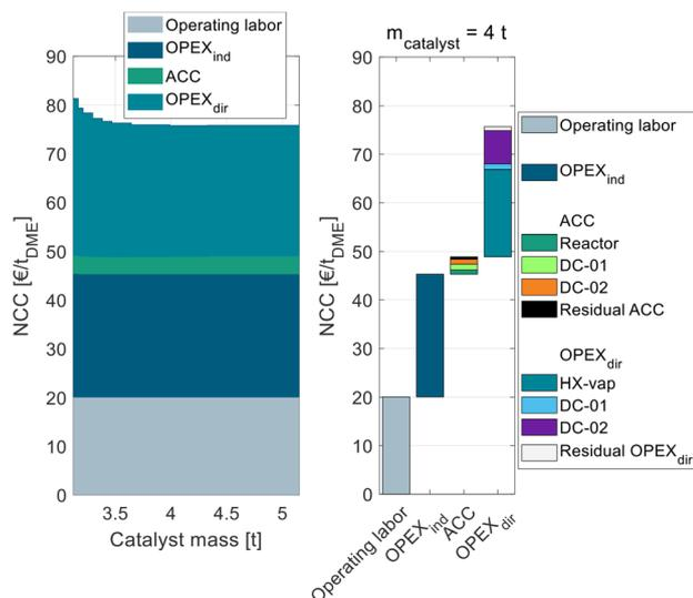
**Fig. 3** Process cost of the conventional process P0 in dependence of the catalyst mass in the conventional gas-phase reactor broken down into ACC, OPEX<sub>ind</sub>, and OPEX<sub>dir</sub>.
