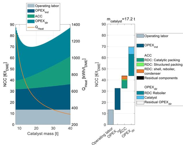
**Fig. 4** Heat demand and NCC of the RD process P2 with C400 and pure MeOH feed in dependence of the catalyst mass in the RDC broken down into ACC, OPEX<sub>ind</sub>, and OPEX<sub>dir</sub> (left) as well as detailed cost breakdown at the cost optimum (right).
