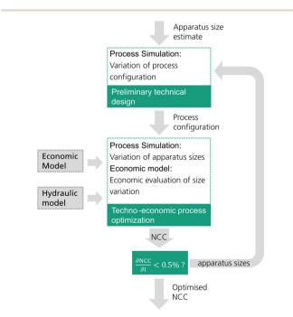
Fig. 2 Methodology of the total cost optimized process design of each process.
