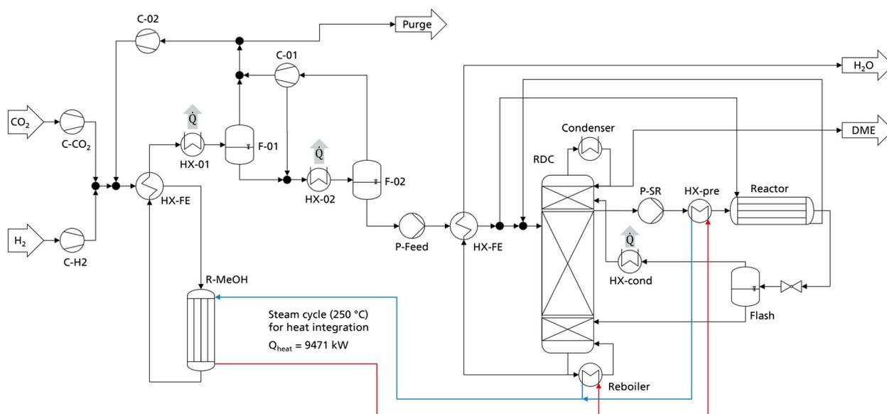
Fig. 8 Flowsheet of the heat integrated MeOH and DME synthesis plant producing DME from CO<sub>2</sub> and H<sub>2</sub>.
