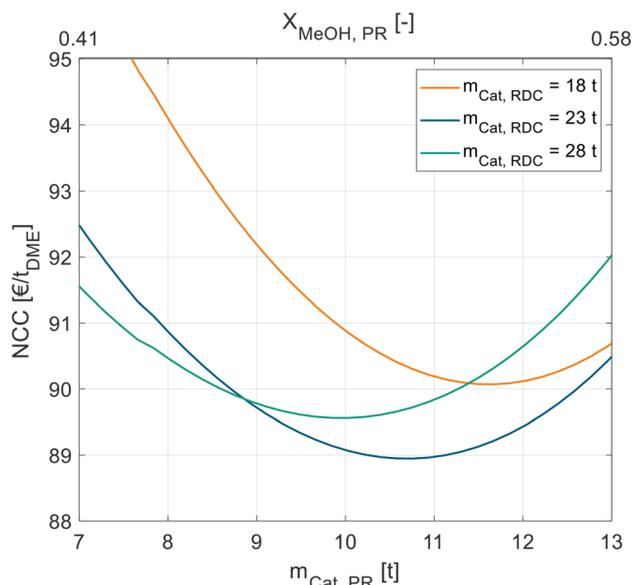
Fig. 5 NCC of process P3 in dependence of the catalyst mass in the liquid-phase PR for different RDC sizes. Exemplary for pure MeOH feed and A36.
