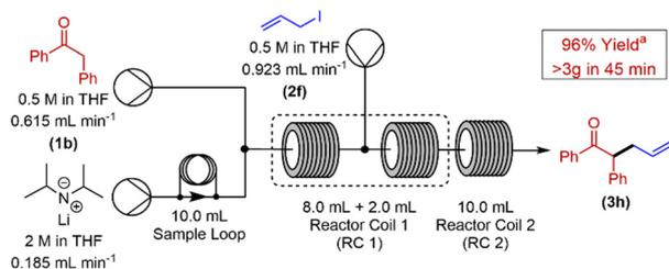
**Scheme 2** Continuous flow set-up for the scale out of 2-phenyl acetophenone  $\alpha$ -allylation. <sup>a</sup>Determined by use of <sup>1</sup>H NMR with 1,3,5-trimethoxybenzene as internal standard.
