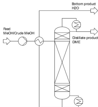
Fig. 3 Process flowsheet used for the process simulation.
