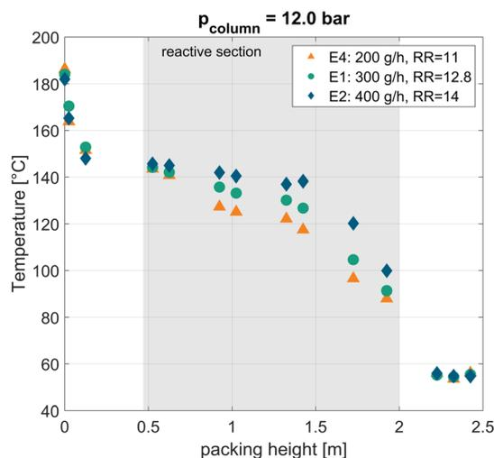
Fig. 5 Measured temperature profiles of the experiments E1, E2 and E4 along the packing height of the column. The feed mass flow is varied and the reflux ratio is adapted in order to achieve a comparable distillate purity.
