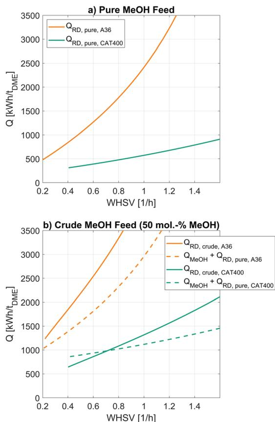
**Fig. 11** Specific reboiler duty per ton of produced DME as a function of the WHSV of the RD column. Comparison between A36 (orange) and Treverlyst CAT 400 (green). Results for pure MeOH feed (top) and crude MeOH feed (bottom) with 50 mol% H<sub>2</sub>O and 50 mol% MeOH.  $N_{rect,upper} = 10$ ,  $N_{rect,lower} = 14$ ,  $N_{reactive} = 25$ .  $N_{Feed} = 10$  in case of pure MeOH feed for both A36 and CAT400. In case of crude MeOH feed  $N_{Feed} = 35$  (A36) or  $N_{Feed} = 25$  (CAT400).
