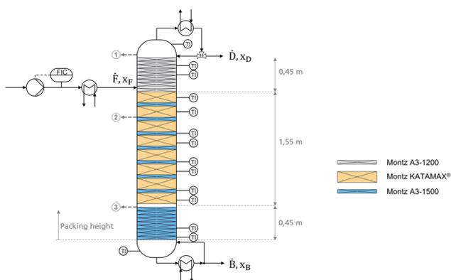
**Fig. 2** Simplified process flow diagram of the pilot reactive distillation setup including positions of sample positions, thermocouples and packed height of the three sections.
