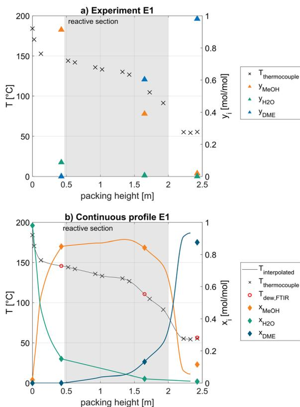
**Fig. 4** a) Discrete measured temperature and gas phase composition along the packing height of the column; b) calculated continuous temperature obtained by interpolation and liquid phase composition obtained from measured gas phase composition according to the methodology described in the simulation chapter; exemplary representation for experiment #1; operating pressure 12.0 bar, feed mass flow 0.3 kg h<sup>-1</sup> pure MeOH.
