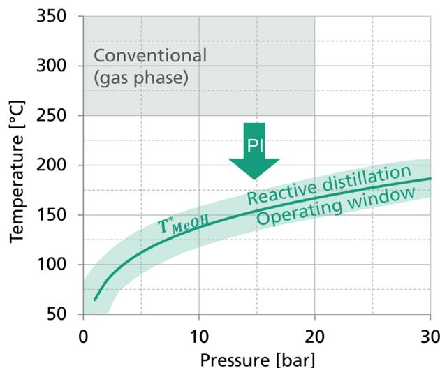
**Fig. 1** Boiling point curve of MeOH and resulting operating window of a process-intensified (PI) reactive distillation process for DME synthesis compared to the operating conditions of the conventional gas phase reaction. Illustration from Gierse *et al.*<sup>16</sup>
