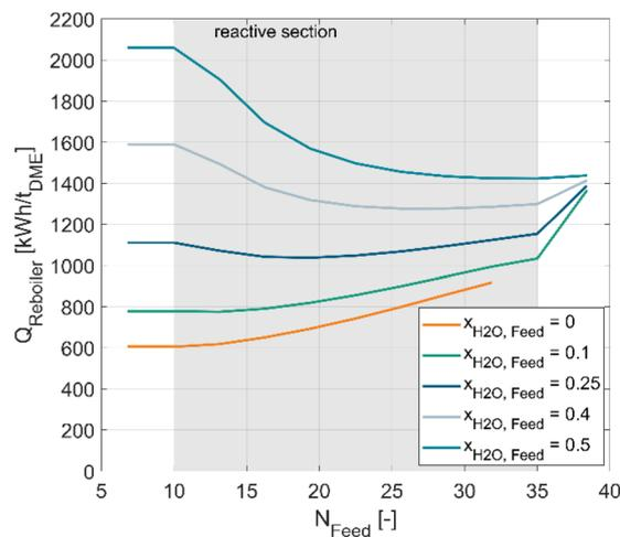
Fig. 10 Specific reboiler duty per ton of produced DME in dependence of the feed stage  $N_{\text{Feed}}$  for various molar water fractions in the feed. WHSV = 0.27.  $N_{\text{rect,upper}} = 10$ ,  $N_{\text{rect,lower}} = 14$ ,  $N_{\text{reactive}} = 25$ . Use of A36 in the reactive section with  $T_{\text{max}} = 130$  °C.
