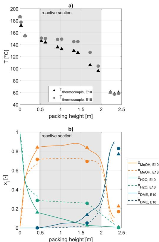
Fig. 6 Comparison of the experiments E10 (pure MeOH feed) and E18 (crude MeOH feed). Measured temperature profile (a) and calculated liquid composition profile (b) of both experiments along the packing height of the column.
