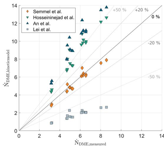
Fig. 7 Measured distillate flow rate  $\dot{N}_{\text{DME,measured}}$  over simulated overall reaction rate  $\dot{N}_{\text{DME,kinetic model}}$  evaluated based on calculated continuous column profiles and different kinetic models.<sup>8,11,16,28</sup> Parity plot for all measured experimental datapoints E1–E18.
