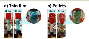
Fig. 2 Using PaDa-I enzyme-loaded hydrogels as (a) a random thin film or (b) pellet packing for continuous flow biocatalysis. The blue color is resulted from trapped ABTS<sup>+</sup> into the hydrogel material.
