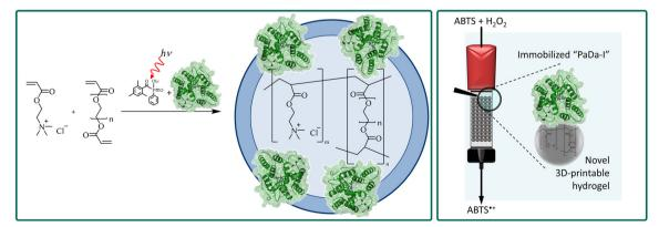
Fig. 1 Concept of this work: synthesis of synthetic 3D printable hydrogels for enzyme immobilization (left). Application of novel heterogeneous enzyme as random packing material for continuous oxyfunctionalization synthesis oxidizing 2,2'-azino-bis(3-ethylbenzothiazoline-6-sulfonic acid) (ABTS).
