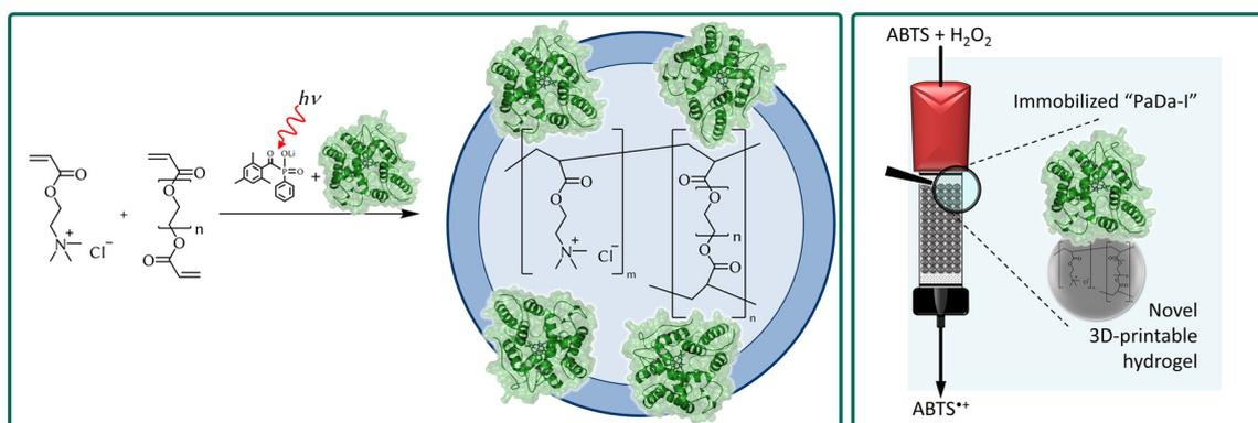
**Fig. 1** Concept of this work: synthesis of synthetic 3D printable hydrogels for enzyme immobilization (left). Application of novel heterogeneous enzyme as random packing material for continuous oxyfunctionalization synthesis oxidizing 2,2'-azino-bis(3-ethylbenzothiazoline-6-sulfonic acid) (ABTS).
