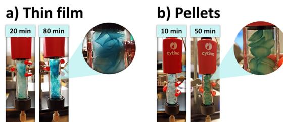
Fig. 2 Using PaDa-I enzyme-loaded hydrogels as (a) a random thin film or (b) pellet packing for continuous flow biocatalysis. The blue color is resulted from trapped  $\text{ABTS}^{++}$  into the hydrogel material.
