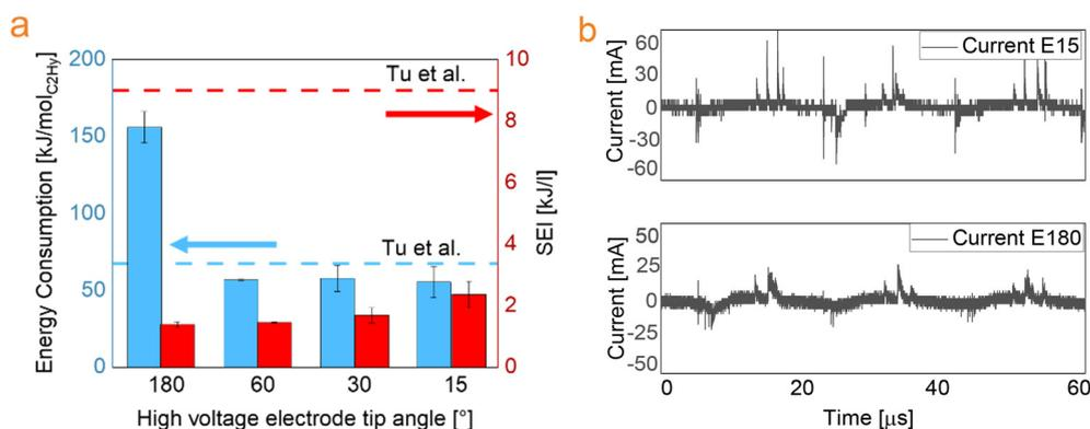
Fig. 5 (a) Effect of HV electrode tip angle on energy consumption and specific energy input (ring electrode length: 3 mm), compared with.<sup>22</sup> (b) Current waveform for the experiments with HV electrode tip angle 15° and 180°.
