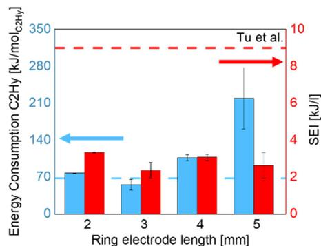
Fig. 11 Energy consumption and specific energy input as a function of ring electrode length.<sup>22</sup>
