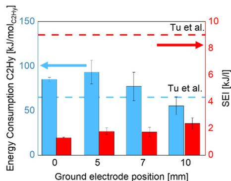
Fig. 7 Energy consumption and specific energy input as a function of the distance between the electrodes.<sup>22</sup>
