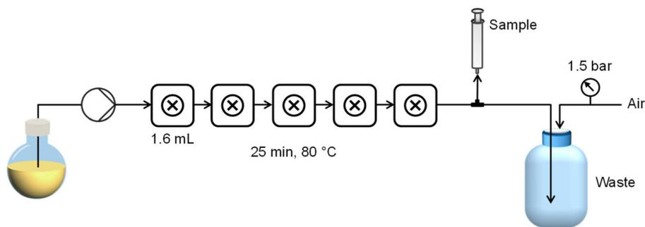
**Fig. 1** Reactor platform for polymer synthesis in a miniature five-CSTR cascade. All five reactors are heated from the same temperature-controlled heating block, with stirring provided by five pairs of neodymium magnets glued to 5 V DC computer fans located underneath the heating block.
