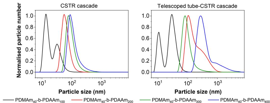
**Fig. 10** Particle size distributions of PDMA<sub>40</sub>-*b*-PDAA<sub>*m*</sub> copolymers prepared via RAFT dispersion polymerisation in a miniature CSTR cascade using a batch macro-CTA (left) versus in a miniature CSTR cascade with a macro-CTA prepared upstream in a telescoped tubular reactor (right). PDMA<sub>40</sub> macro-CTA was prepared at 80 °C for 40 minutes, with copolymerisation at 70 °C for 50 minutes. [CTA] : [initiator] = 10 : 1.
