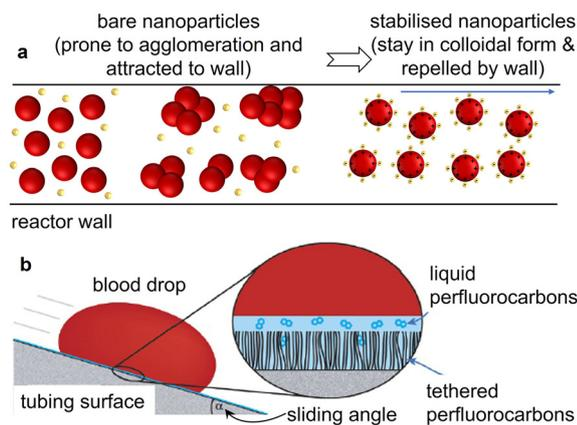
**Fig. 4** (a) Schematic illustration of particle stabilisation helping in fouling resistance. (b) Schematic of repellence characteristics of SLIPS antifouling coatings (tethered perfluorocarbon in the porous surface and liquid perfluorocarbon forming a stable film on top) (reproduced from ref. 81 with permission from Springer, © 2014).
