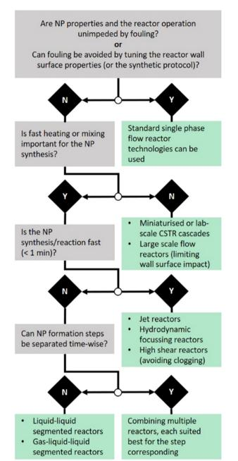
Fig. 11 Decision tree of guidelines to design non-fouling flow reactors.
