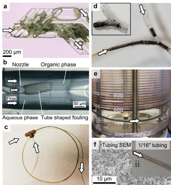
**Fig. 1** Flow reactors that fouled during the synthesis of (a) silver,<sup>35</sup> (b) lipid,<sup>36</sup> (c) iron oxide,<sup>37</sup> (d) palladium,<sup>18</sup> (reproduced from ref. 18 and 35–37 with permission from the Royal Society of Chemistry, © 2017, 2015, 2021 & 2023) and (e and f) gold nanoparticles (reproduced from ref. 38 and 39 with permission from Elsevier, © 2022 & 2018).
