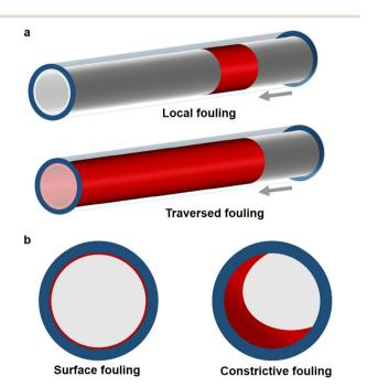
Fig. 2 Fouling classification in tubular reactors considering (a) axial and (b) radial characteristics.
