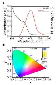
Fig. 4 (a) UV-vis absorption, PL spectrum and (b) CIE 1931 color space chromaticity diagram of InP/ZnS QDs synthesized in our continuous flow setup. The inset in (b) shows the photograph of the corresponding InP/ZnS QDs colloid solution under 356 nm UV irradiation and PLQY.
