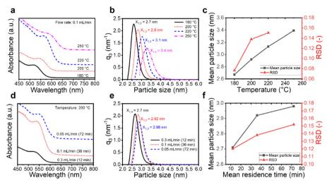
Fig. 3 (a and d) UV-vis absorption spectra, (b and e) corresponding PSDs and (c and f) mean particle size and RSD of InP QDs synthesized at different temperatures and flow rates. Experimental conditions: a-c at 0.1 mL min<sup>-1</sup> and 180-250 °C; d-f at 200 °C and 0.05-0.3 mL min<sup>-1</sup>.
