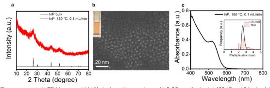
Fig. 2 (a) XRD measurement, (b) TEM image and (c) UV-vis absorption spectrum of InP QDs synthesized at 180 °C and 0.1 mL min<sup>-1</sup>. The inset in (b) shows the InP QD dispersion obtained after washing and the inset in (c) shows the direct comparison of the PSD derived from the UV-vis data and the PSD derived from TEM (101 particles were analysed and evaluated by ImageJ).
