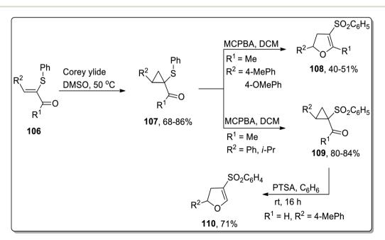
Scheme 33 Synthesis of 2,3-dihydrofurans 110 and cyclopropyl sulfones 108 via Cloke-Wilson rearrangement.
