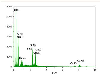
Fig. 4 EDS analysis of [DABCO](SO<sub>3</sub>H)<sub>2</sub>CuCl<sub>4</sub>.
