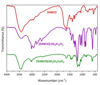
Fig. 1 FT-IR spectra of DABCO, [DABCO]( $SO_3H$ )<sub>2</sub>Cl<sub>2</sub> and [DABCO]( $SO_3H$ )<sub>2</sub>CuCl<sub>4</sub>.
