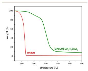
Fig. 2 TGA curves of DABCO and [DABCO](SO<sub>3</sub>H)<sub>2</sub>CuCl<sub>4</sub>
