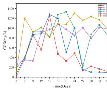
Fig. 4 Changes in COD concentration in different reactors (in mono-digestion C: control reactor; CA: nano- $\text{Al}_2\text{O}_3$  reactor; CC: MWCNTs reactor; in co-digestion CT: control reactor; CTA: nano- $\text{Al}_2\text{O}_3$  reactor; CTC: MWCNTs reactor).
