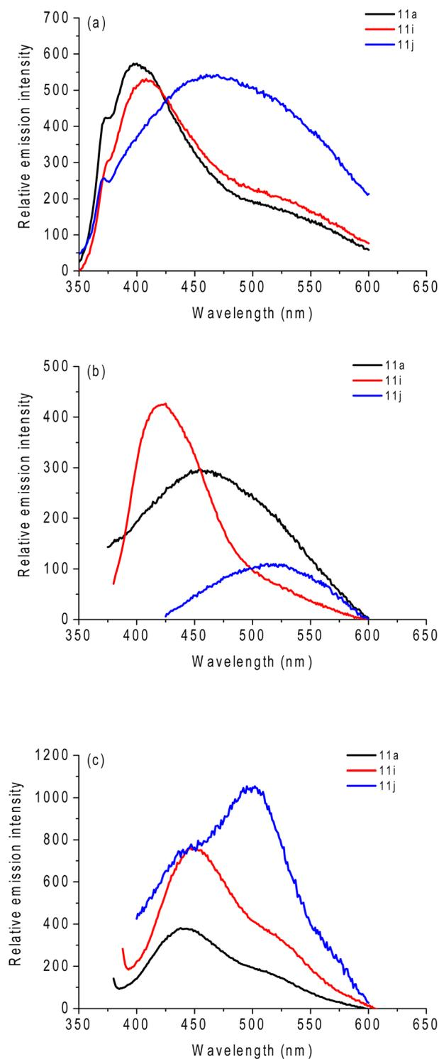
Fig. 4 Comparative steady-state fluorescence emission spectra (concentration at 5.0  $\mu\text{M}$ ) of compounds **11a** (Se atom), **11i** (S atom) and **11j** (Te atom) in (a) DCM, (b) ACN and (c) DMSO, respectively. The compounds were excited in the higher energy transition band.
