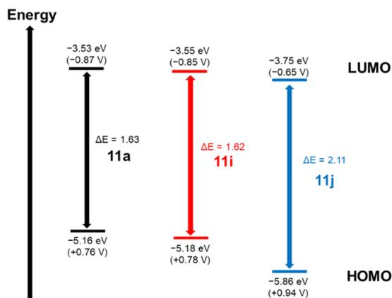
Fig. 6 Comparative redox potentials (*versus* SHE) by HOMO and LUMO levels (in eV) determined by cyclic voltammetry analysis of compounds **11a**, **11i** and **11j** in DCM solution using TBAPF<sub>6</sub> as the supporting electrolyte.
