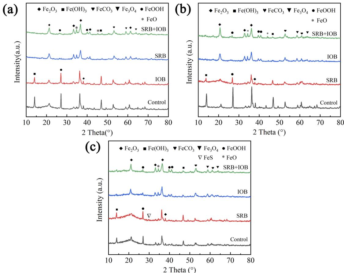
Fig. 2 Corrosion product compositions of X80 pipeline steel in microbial environments at different times: (a) 3 days, (b) 6 days, (c) 15 days.
