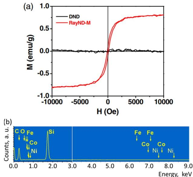
Fig. 10 Magnetic properties of RayND-M ( $d = 4.3-4.5$  nm). (a) Magnetization curve of RayND-M [in comparison with ordinary detonation ND (DND),  $d = 3-10$  nm]. (b) EDS spectrum of RayND-M; Fe, Co, and Ni atoms as impurities were not detected.<sup>139</sup> Reproduced with permission from ref. 139 Copyright 2018 SPIE.
