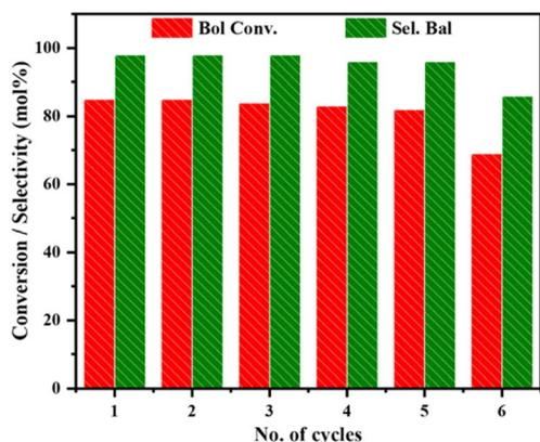
Fig. 13 Catalyst recycling study for the oxidation of benzyl alcohol using the  $\text{WO}_x/\text{CeO}_2\text{-SiO}_2$  (W/CeSi) catalyst. Reaction conditions: 10 wt% of catalyst, 5 mmol of benzyl alcohol,  $\text{O}_2$  bubbling ( $20 \text{ mL min}^{-1}$ ),  $140^\circ\text{C}$  of temperature, 4 h of reaction time, and 800 rpm of stirring speed.
