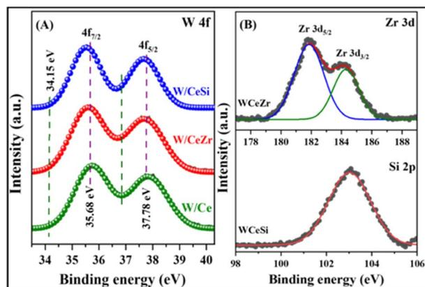
Fig. 7 XPS patterns of the (A) W 4f spectra, and (B) Zr 3d and Si 2p spectra of  $\text{WO}_x/\text{CeO}_2$  (W/Ce),  $\text{WO}_x/\text{CeO}_2\text{-ZrO}_2$  (W/CeZr), and  $\text{WO}_x/\text{CeO}_2\text{-SiO}_2$  (W/CeSi) oxide samples.
