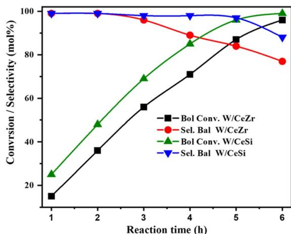
Fig. 10 The effect of the reaction time on the catalytic oxidation of benzyl alcohol over  $WO_x/CeO_2-ZrO_2$  (W/CeZr), and  $WO_x/CeO_2-SiO_2$  (W/CeSi) catalysts. Reaction conditions: 10 wt% of catalyst, 5 mmol of benzyl alcohol,  $O_2$  bubbling ( $20\text{ mL min}^{-1}$ ),  $140\text{ }^\circ\text{C}$  of temperature, and 800 rpm of stirring speed.
