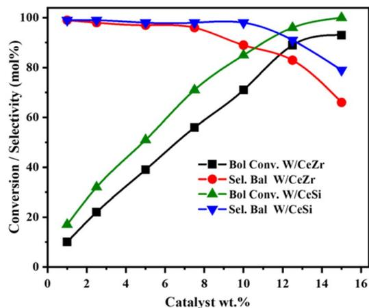
Fig. 12 The effect of catalyst loading on the catalytic oxidation of benzyl alcohol over  $\text{WO}_x/\text{CeO}_2\text{-ZrO}_2$  (W/CeZr), and  $\text{WO}_x/\text{CeO}_2\text{-SiO}_2$  (W/CeSi) catalysts. Reaction conditions: 5 mmol of benzyl alcohol,  $\text{O}_2$  bubbling ( $20 \text{ mL min}^{-1}$ ),  $140^\circ\text{C}$  of temperature, 4 h of reaction time, and 800 rpm of stirring speed.
