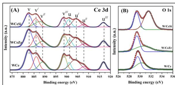
Fig. 6 XPS patterns of (A) Ce 3d spectra, and (B) O 1s spectra for  $\text{WO}_x/\text{CeO}_2$  (W/Ce),  $\text{WO}_x/\text{CeO}_2\text{-ZrO}_2$  (W/CeZr), and  $\text{WO}_x/\text{CeO}_2\text{-SiO}_2$  (W/CeSi) samples.
