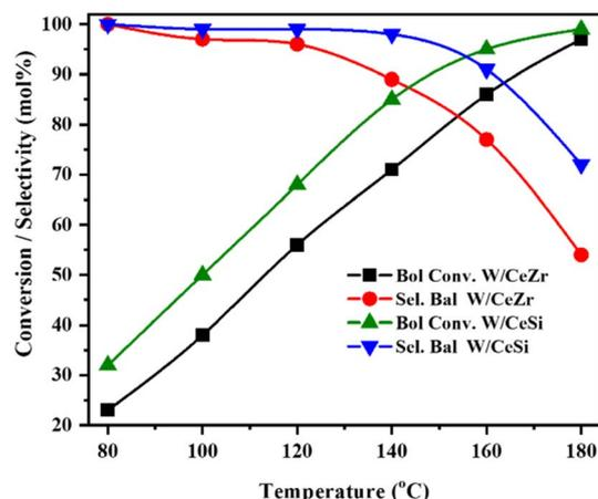
Fig. 11 The effect of temperature on the catalytic oxidation of benzyl alcohol over  $WO_x/CeO_2-ZrO_2$  (W/CeZr) and  $WO_x/CeO_2-SiO_2$  (W/CeSi) catalysts. Reaction conditions: 10 wt% of catalyst, 5 mmol of benzyl alcohol,  $O_2$  bubbling ( $20\text{ mL min}^{-1}$ ), 4 h of reaction time, and 800 rpm of stirring speed.
