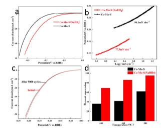
Fig. 4 (a) LSV curves of HER for Co–Mo–S and Co–Mo–S (NaBH<sub>4</sub>). (b) Tafel plots of Co–Mo–S and Co–Mo–S (NaBH<sub>4</sub>). (c) Polarization curve of Co–Mo–S (NaBH<sub>4</sub>) catalyst before and after 5000 CV cycles. (d) Conversion of thiophene over Co–Mo–S and Co–Mo–S (NaBH<sub>4</sub>) towards HDS at different temperatures.
