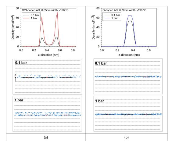
Fig. 14 Local density distributions in z-direction and snapshots of  $H_2$  adsorption in (a) O/N-doped AC model (0.85 nm width) and (b) O-doped AC model (0.70 nm width) at -196 °C.
