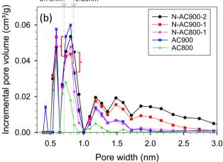
Fig. 3 (a)  $N_2$  adsorption/desorption isotherms at -196 °C and (b) pore size distributions.
