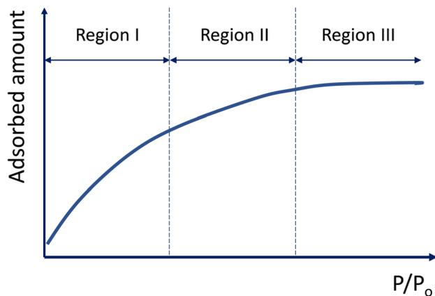
Fig. 8 Adsorption process with increasing relative pressure.
