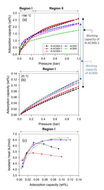
Fig. 9  $\,$  H $_2$  adsorption isotherms at (a) -196 and (b) 25  $\,^{\circ}$ C up to 1 bar, and (c) isosteric heat.
