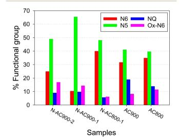
Fig. 7 Comparison of nitrogen functional group species on AC samples obtained from XPS.
