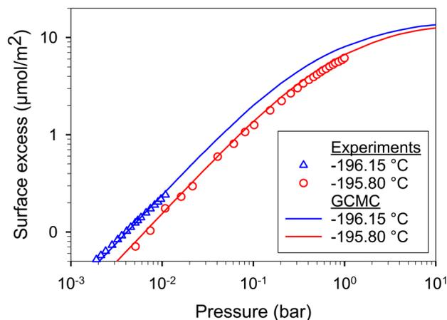
Fig. 11 H<sub>2</sub> adsorption on graphite surface at  $-196.15$  and  $-195.80$  °C obtained with GCMC (this work) and experimental data.<sup>67,68</sup>
