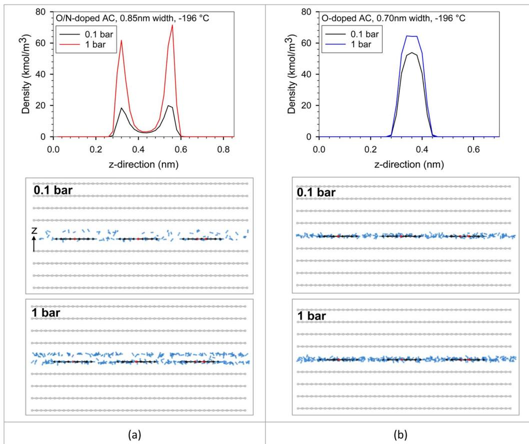
Fig. 14 Local density distributions in z-direction and snapshots of H<sub>2</sub> adsorption in (a) O/N-doped AC model (0.85 nm width) and (b) O-doped AC model (0.70 nm width) at  $-196$  °C.
