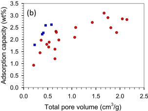
Fig. 10  $\,$  H<sub>2</sub> adsorption capacity *versus* (a) specific surface area and (b) pore volume obtained with the present work and literature (other works) at -196 °C and 1 bar corresponding to Table 1.
