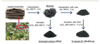
Fig. 1 Synthesis of the original and modified ACs.
