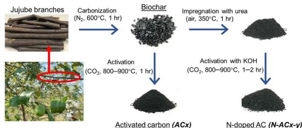
Fig. 1 Synthesis of the original and modified ACs.
