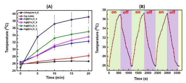
Fig. 4 (A) Temperature changes of Ag nanocubes, Ag@Cu<sub>2</sub>O hybrid nanoparticles colloidal solutions synthesized adding (a)10  $\mu$ L, (b)20  $\mu$ L, (c) 30  $\mu$ L, (d) 40  $\mu$ L of 0.1 M Cu(NO<sub>3</sub>)<sub>2</sub> and water over time under irradiation with the NIR laser at 808 nm. (B) Photothermal stability test of Ag@Cu<sub>2</sub>O\_d exposed to 808 nm laser irradiation for three cycles.
