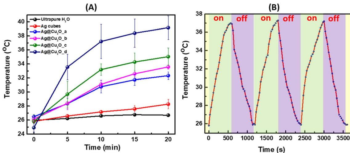
Fig. 4 (A) Temperature changes of Ag nanocubes, Ag@Cu<sub>2</sub>O hybrid nanoparticles colloidal solutions synthesized adding (a) 10  $\mu$ L, (b) 20  $\mu$ L, (c) 30  $\mu$ L, (d) 40  $\mu$ L of 0.1 M Cu(NO<sub>3</sub>)<sub>2</sub> and water over time under irradiation with the NIR laser at 808 nm. (B) Photothermal stability test of Ag@Cu<sub>2</sub>O<sub>d</sub> exposed to 808 nm laser irradiation for three cycles.
