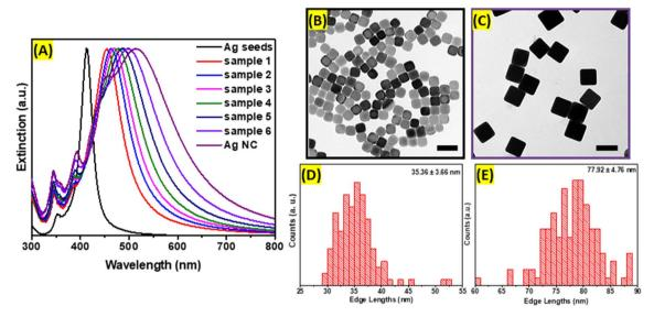
Fig. 1 (A) Extinction spectra measured during the seed-mediated overgrowth of Ag nanocubes. TEM images of (B) cubic Ag seeds and (C) large Ag cubes. Scale bars: 100 nm. Size distributions of the edge lengths of (D) cubic Ag seeds and (E) large Ag cubes.
