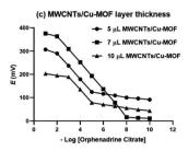
Fig. 6 The effect of the ion-to-electron transducer layer on the potentiometric response of the GCE, (a) Cu-MOF, (b) MWCNTs and (c) MWCNTs/Cu-MOF composite.
