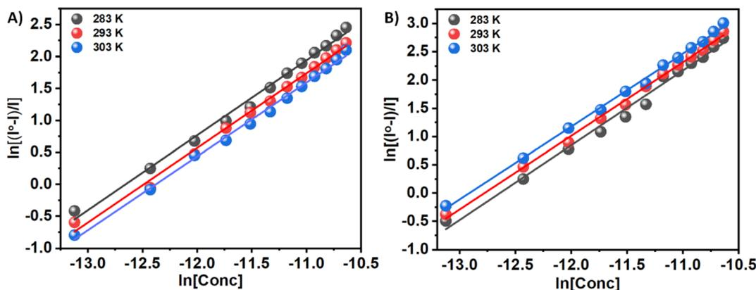
Fig. 4  $\ln((I^0 - I)/I)$  versus  $\ln[C]$  plots for the quenching of Tyr-fluorescence of insulin at 283, 293, and 303 K in the presence of two Schiff base **3a** (Panel A) and **3b** (Panel B) in solution.
