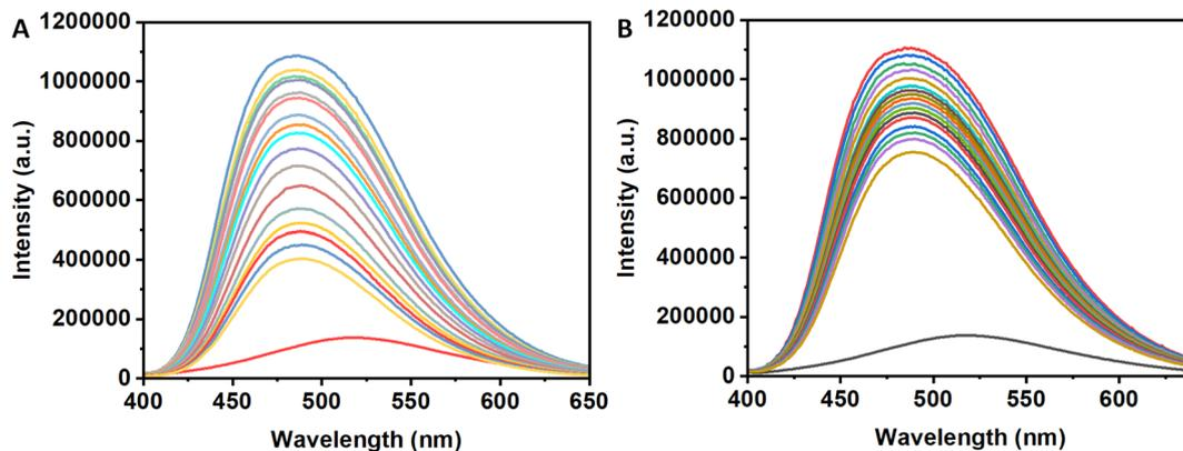
Fig. 6 ANS-fluorescence emission spectra of monomeric insulin incubated separately at 25 °C and at pH 2.0 in the absence and presence of Schiff base **3a** (Panel A) and in the absence and presence of Schiff base **3b** (Panel B). Insulin concentrations throughout all the experiments were kept at 25  $\mu\text{M}$ . Results were the average of three different experiments.
