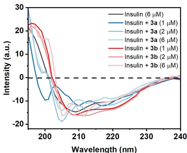
Fig. 7 Far-UV CD spectra (190–250 nm) of monomeric insulin in the absence and presence two small molecules (Schiff bases) **3a** and **3b** at 25 °C and at pH 2.0, showing the secondary structural changes of insulin.
