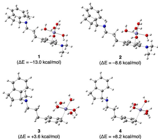
Fig. 5 Optimized geometries of hydrated iron-GIF-2197-r (1), GIF-2027 (2), GIF-2228-r (3), and GIF-2227-r (4) complexes. The most stable complexes of  $\text{Fe}(\text{OH}_2)_6^{2+}$  with GIF compounds are shown.  $\Delta E$  represents the complex stabilization energy ( $\text{kcal mol}^{-1}$ ). In racemate GIF complexes, the  $\Delta E$  value corresponds to that of the *R*-form.
