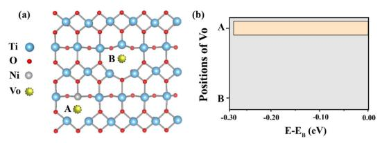
Fig. 1 (a) Two possible positions of the oxygen vacancy in the Ni doped  $TiO_2$  structure. For position A, the oxygen vacancy is near the Ni, whereas this vacancy does not interact with the Ni when it is located at position B. (b) Total energy corresponds to two positions of the oxygen vacancy.
