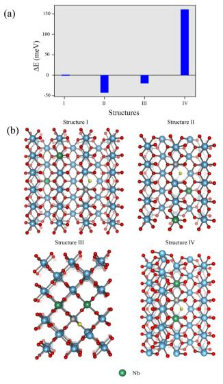
Fig. 2 (a) Total energy of two Nb atoms in the  $TiO_2$  with  $NiV_o$  inside. (b) Four different positions of Nb in the Ni doped  $TiO_2$ : structure I, two Nb atoms are isolated from both Ni and  $V_o$ . Structures II and III, two Nb atoms approach the  $V_o$  and Ni sides, respectively. Structure IV, Ni and two Nb atoms form as a Nb<sub>2</sub>Ni chain.
