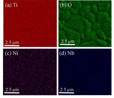
Fig. 7 SEM mapping images of 2.5%NiNTO for (a) Ti, (b) O, (c) Ni, and (d) Nb elements.
