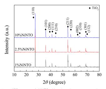
Fig. 4 XRD patterns of xNiNTO with various dopant concentrations.
