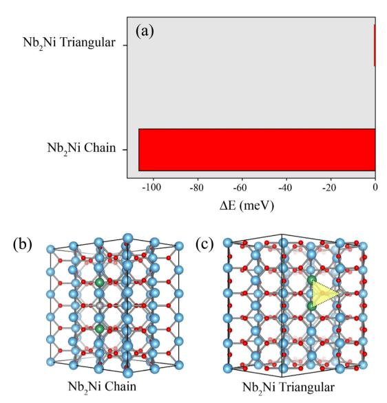
Fig. 3 (a) Total energy associated with Nb<sub>2</sub>Ni in two distinct configurations. (b) Chain configuration of Nb<sub>2</sub>Ni. (c) Triangular configuration of Nb<sub>2</sub>Ni.
