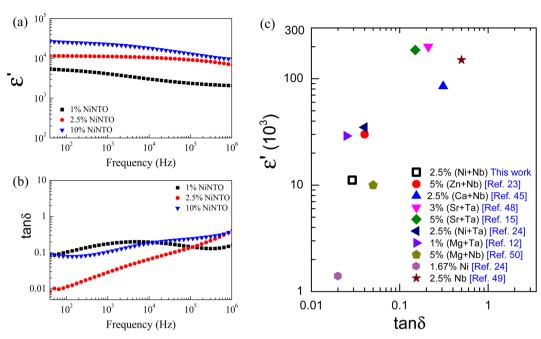
Fig. 8 Frequency dependence of dielectric properties of (a)  $\varepsilon'$  and (b)  $\tan\delta$  at  $\sim$ 30 °C for 1%NiNTO, 2.5%NiNTO, and 10%NiNTO. (c)  $\varepsilon'$  and  $\tan\delta$  at  $\sim$ 30 °C and 1 kHz of 2.5%NiNTO compared to previous works.
