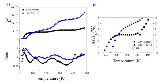
Fig. 9 (a) Temperature-dependent behaviors of  $\varepsilon'$  and  $\tan \delta$  for ceramics composed of 2.5%NiNTO and 10%NiNTO, measured over a temperature range of 20 to 483 K. (b) Temperature coefficient of  $\varepsilon'$  at a frequency of 1 kHz for 2.5%NiNTO and 10%NiNTO.
