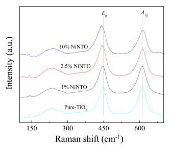
Fig. 5 Raman spectra of  ${\rm TiO_2}$  and  $x{\rm NiNTO}$  with various dopant concentrations.
